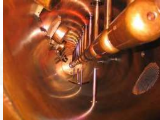
Inside Drift Tube Tank
