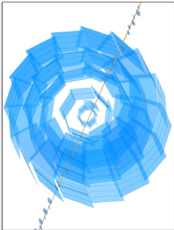
Very good consistency with previous alignment data but bowing of L2 ladders slightly increased after installation
