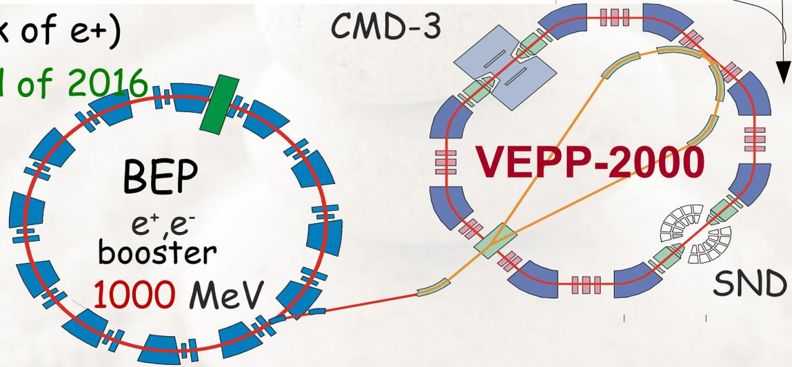
Maximum c.m. energy is 2 GeV, project luminosity is  $L = 10^{32} \text{ cm}^{-2} \text{ s}^{-1}$  at  $2E = 2 \text{ GeV}$
