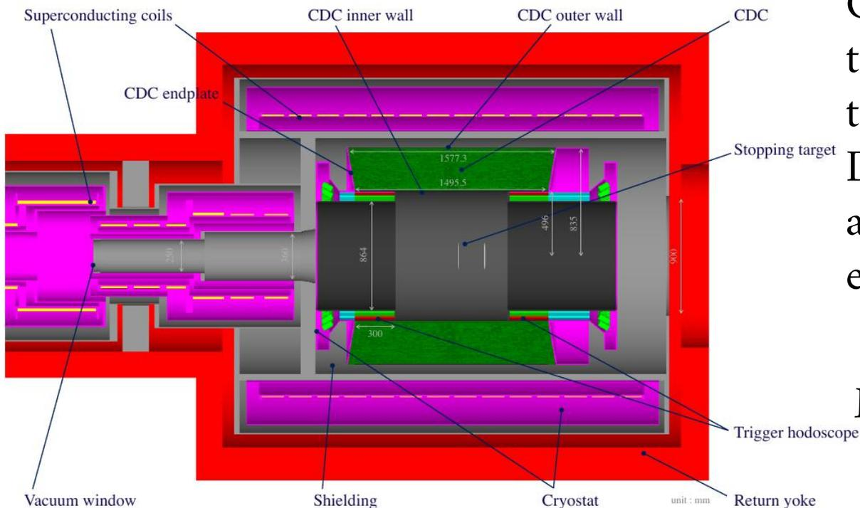
CyDet is located after the bridge solenoid in the muon transport section, and installed inside the warm bore of a large 1 T superconducting Detector Solenoid . The CyDet must accurately and efficiently identify and measure 105 MeV electrons whilst rejecting backgrounds.
