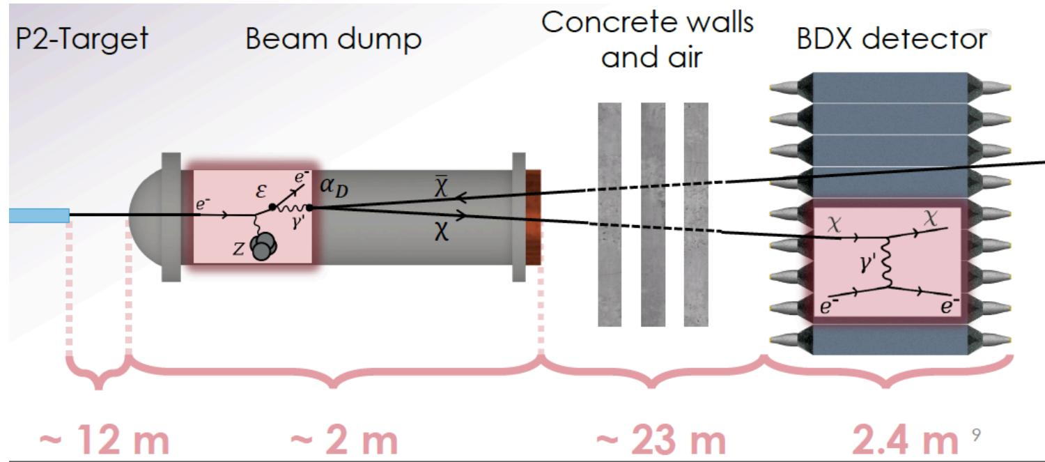
**Electron Scattering (MESA) on Beam Dump
