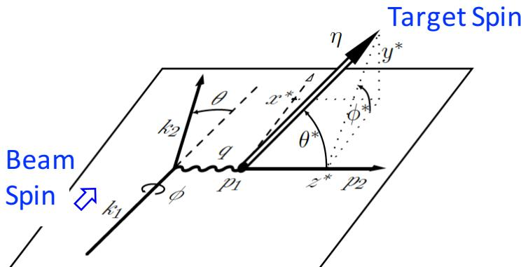
$$\left. \begin{array}{l} \phi^* = 0 \\ \theta^* = 0, \frac{\pi}{2} \end{array} \right\} \Rightarrow A_{\perp} \sim \frac{G_E}{G_M}$$
