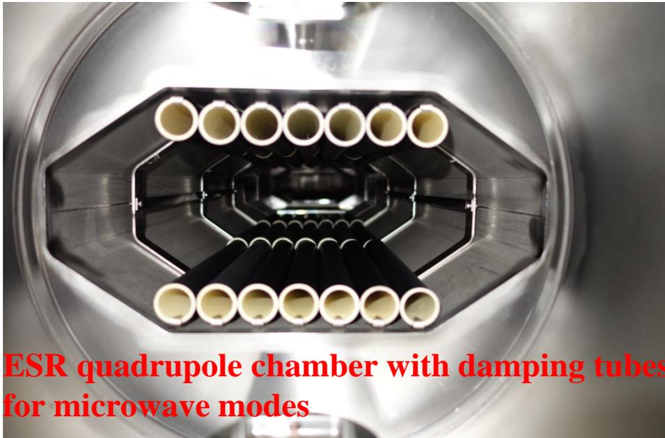
**ESR quadrupole chamber with damping tubes for microwave modes**
