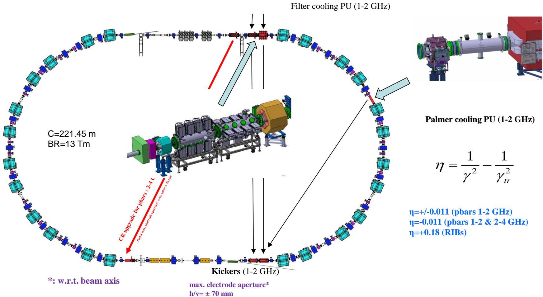
The CR is designed to have required  $\eta$  parameter both for antiprotons and RIBs. Optics and positions of PU and KI are designed for the required dispersion & phase advances between all pairs of PU-KI. The size of all beams must be smaller than the specified internal apertures of the electrodes at PU/KI.
