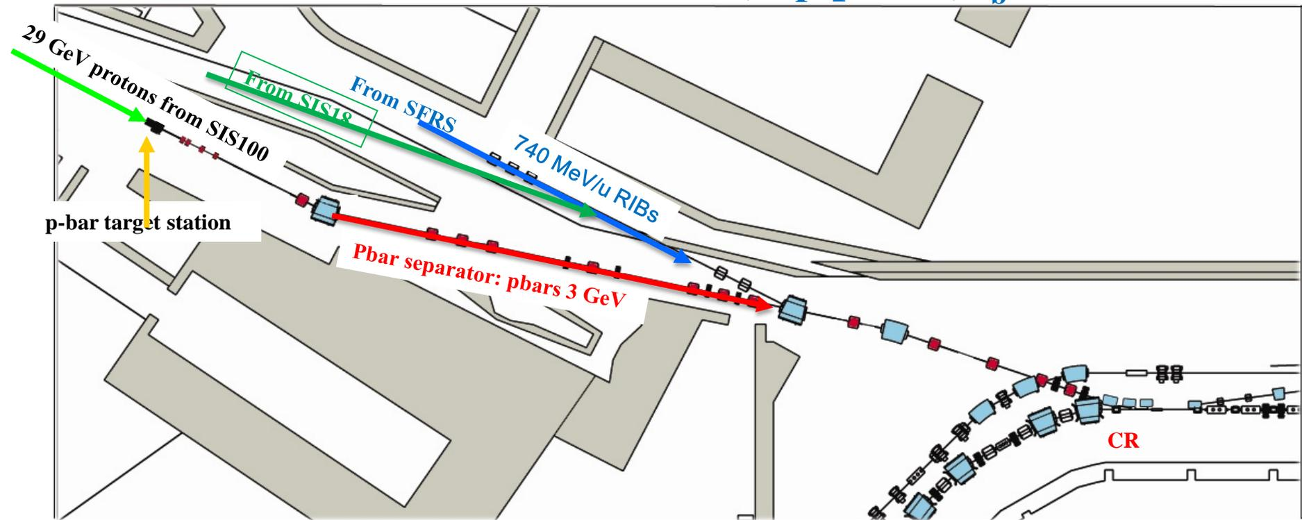
Antiprotons from pbar-sep.:  $240 \pi$  mm\*mrad;  $\Delta p/p=6\%$ ;  $t_b=50$  ns
