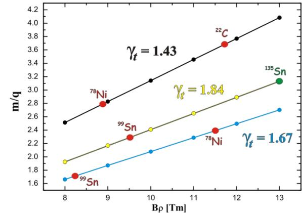
$$\frac{\Delta f}{f} = -\frac{1}{\gamma_{tr}^2} \frac{\Delta(m/q)}{m/q} + \left(1 - \frac{\gamma^2}{\gamma_{tr}^2}\right) \frac{\Delta v}{v} + \left(\frac{\delta f}{f}\right)_{error}$$
