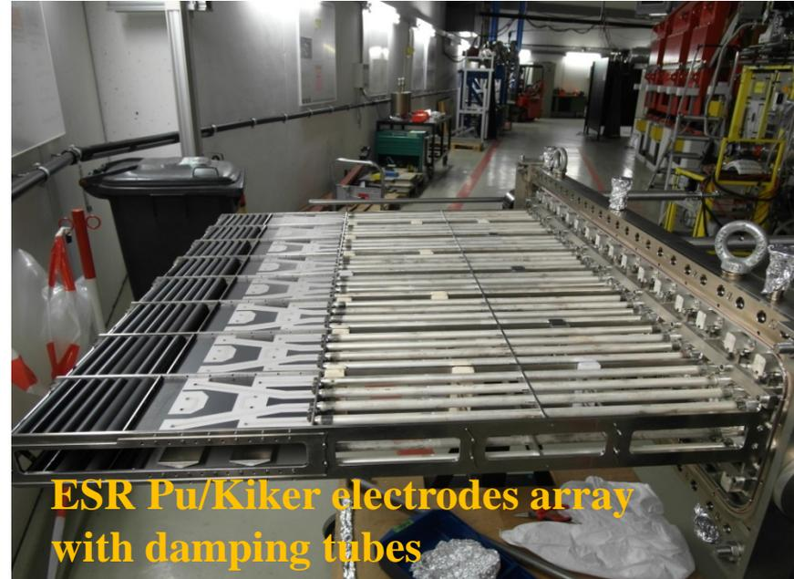
**ESR Pu/Kiker electrodes array with damping tubes**
