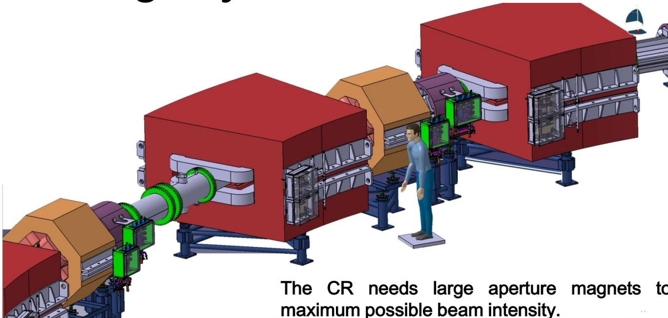
The CR needs large aperture magnets to collect the maximum possible beam intensity.
