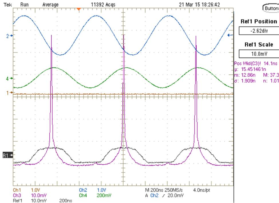
RF of 1<sup>st</sup> harmonic and Phase probe signal of p-beam
