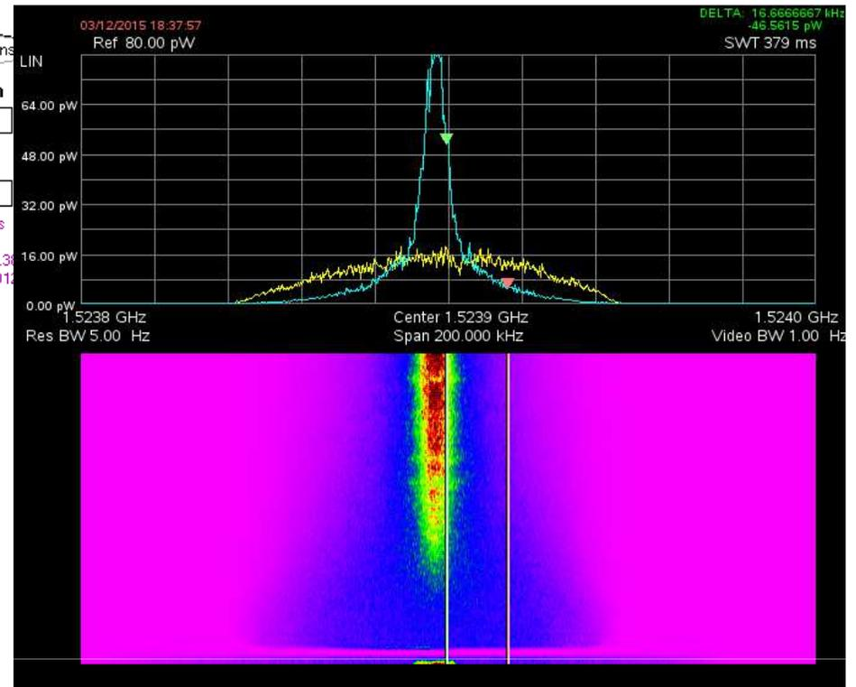
RF on, e-cooling with 550 mA, final  $\Delta p/p = 10^{-4}$
