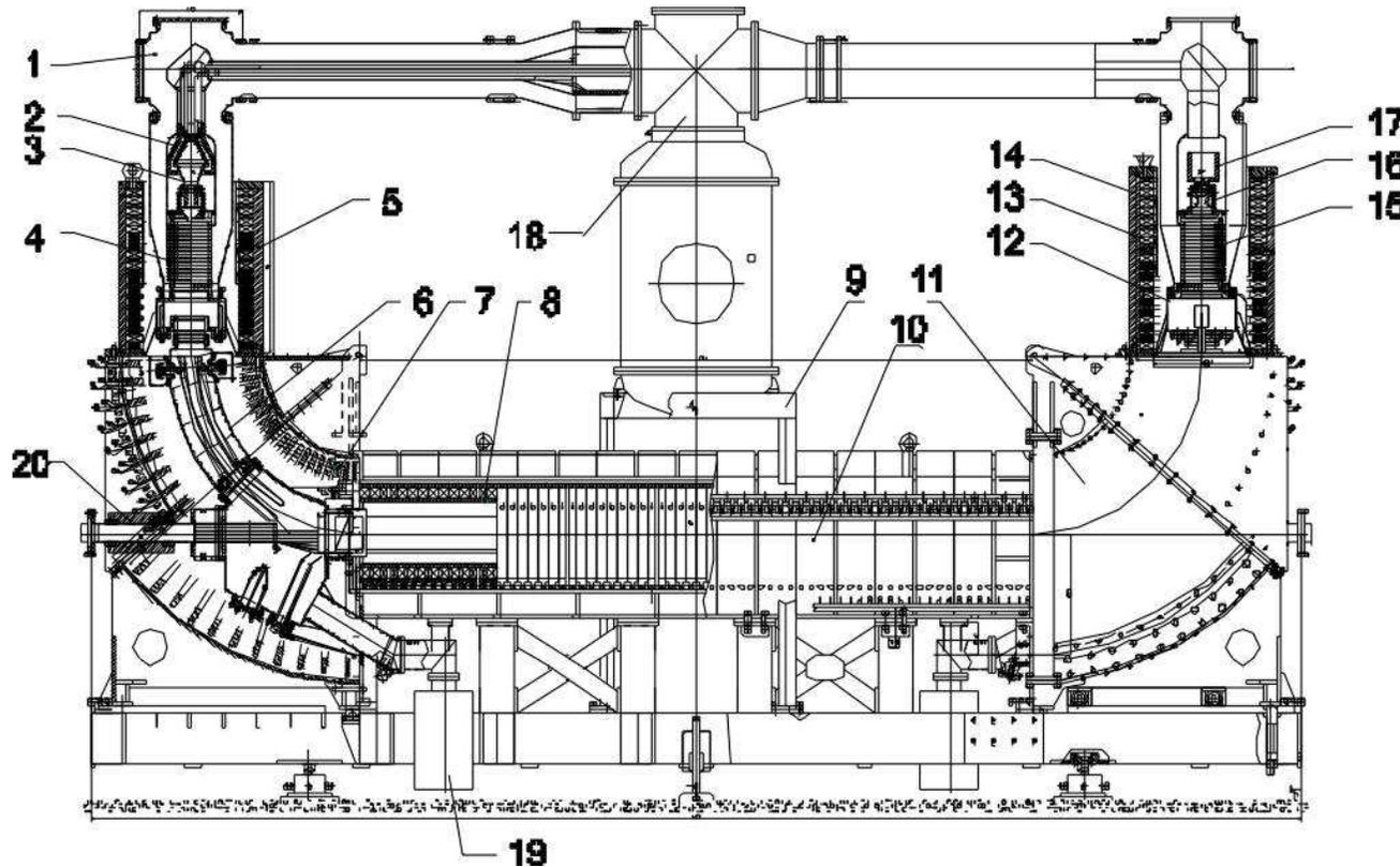
EC-300 electron cooler for CSRe storage ring (Lanzhou, China)
