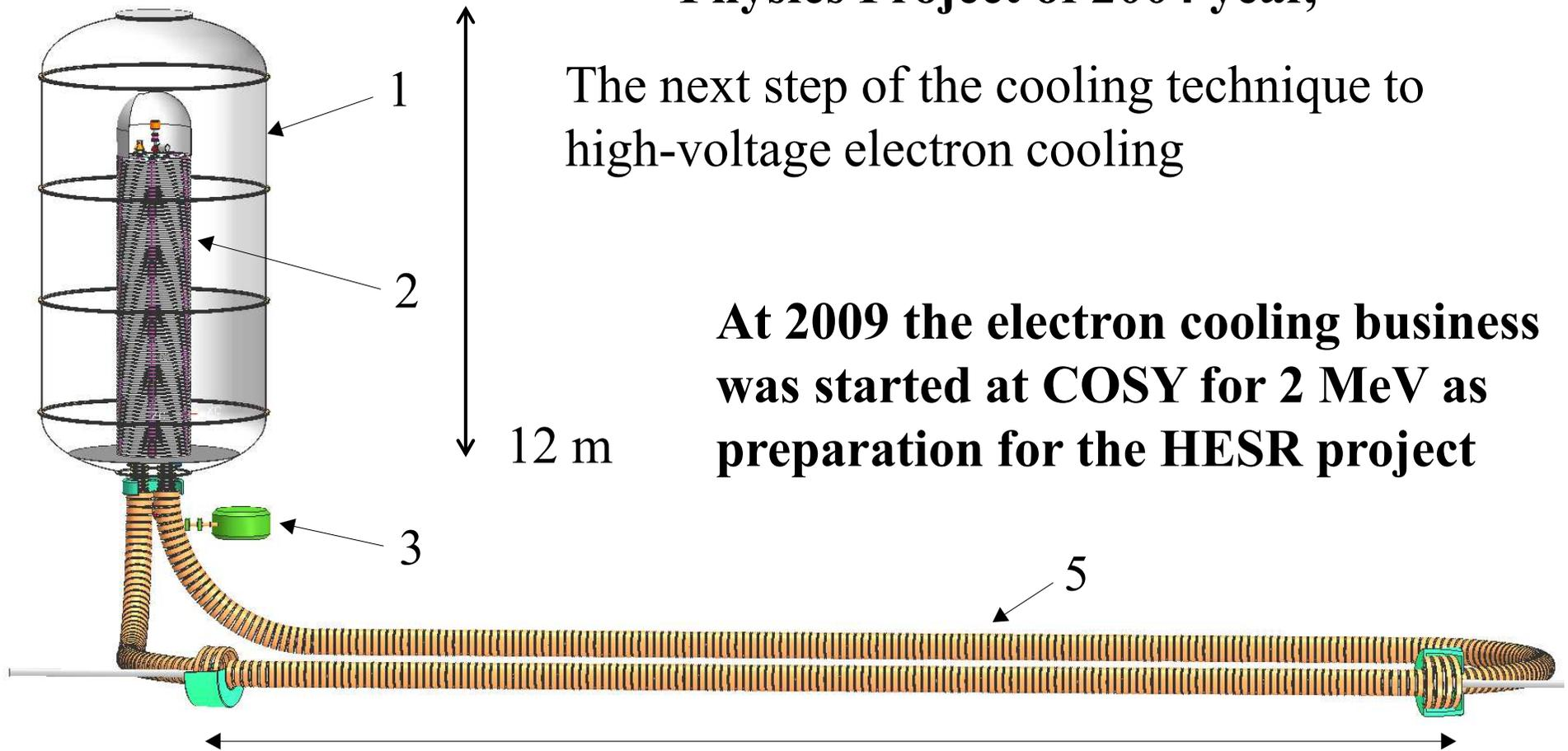
1 – high voltage tank; 2 – electrostatic column; 3 – cyclotron for charging of the head of electrostatic column; 4 – cooling section (30 m); 5 – reversal track.
