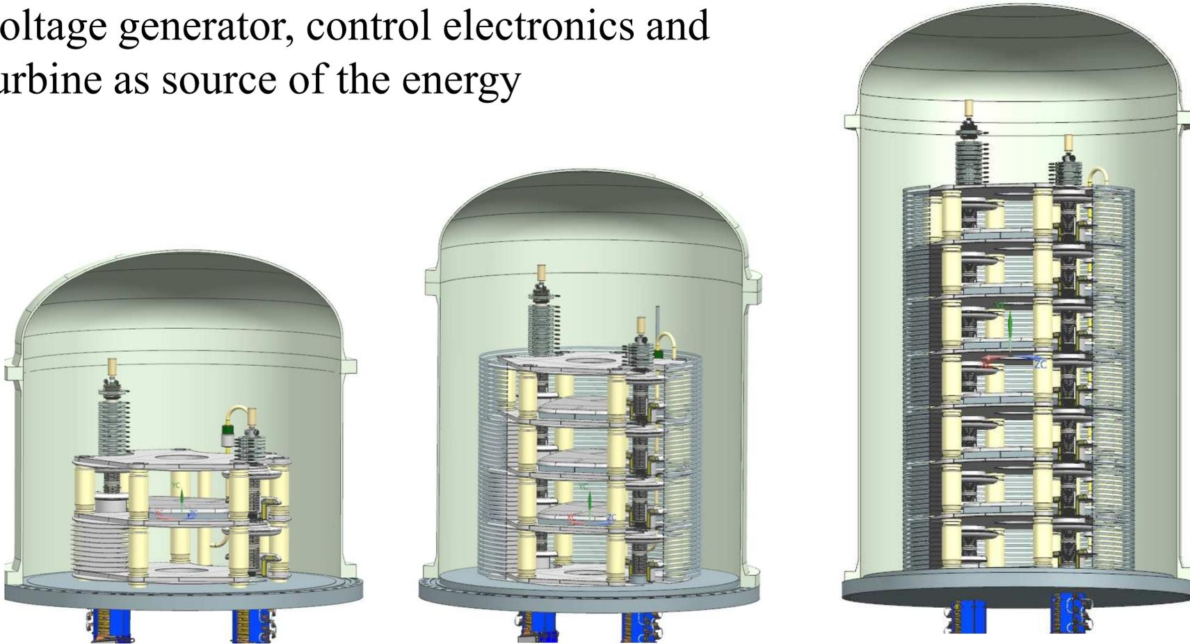
Sequence of designs of the high-voltage tanks for 1, 2 and 4 MeV. The design of the bottom is identical. So, the transport channel may be identical too. The size of the bottom is enough for the construction of 8 MeV cooler also.
