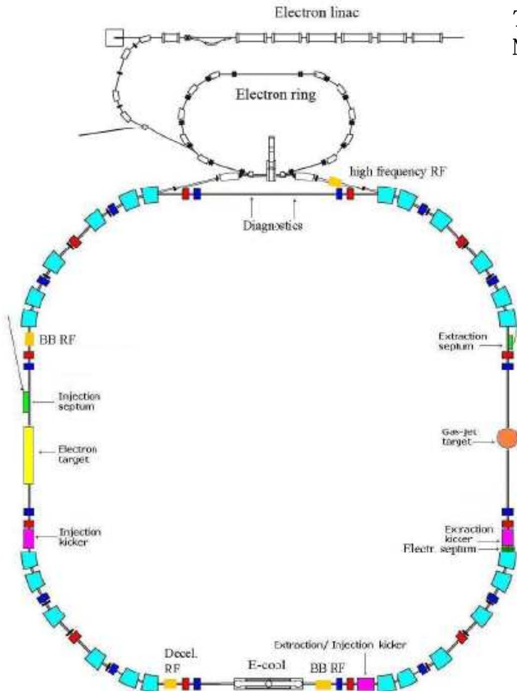
The New Experimental Storage Ring NESR with its instrumentation for atomic physics experiments
