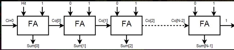
Delay line is realised with Full Adders [3]
