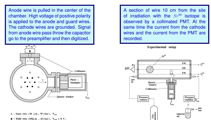
For cathode aging measurements the drift cell was irradiated with the  $Sr^{90}$  isotope and the accumulated charge was measured per unit length of the anode wire in mC/cm. When the Malter current appeared its time dependence is measured. In the event of Malter emission it was discovered 30 seconds delay in the current rise from the PMT relative to the current rise from the wires.
