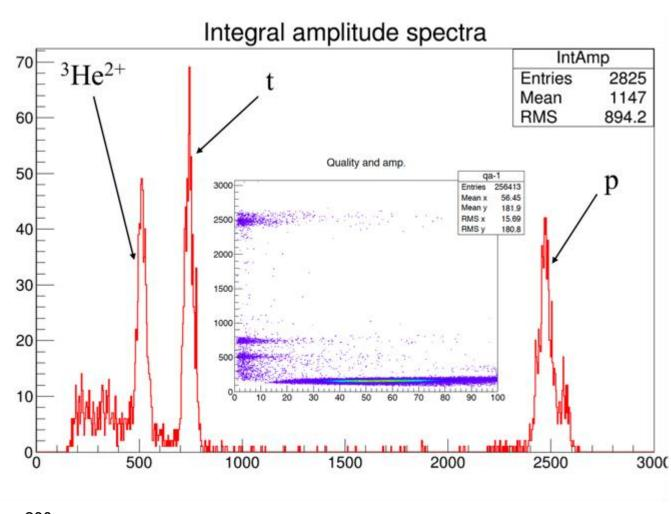
In the test-run of 2015 the foil of deuterated polymethylmetacrylate was used as a target. The reaction products energy measured by eight silicon detectors that surrounded the collision area.
