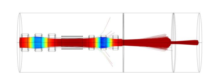
The new focusing system consists of two einzel lenses and the deflector.
