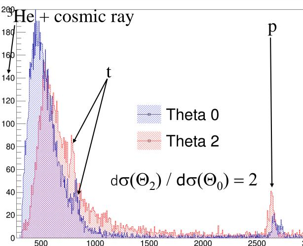
Results of the test-run in 2019 with heavy water vapor  $(D_2O)$ as  $(\sim 10^{18} \text{ atoms/}_{\text{s}})$ . POLIS provided the ion beam of 10 μA with 10 keV energy. The  $4 \pi$  detector system had 22 silicon detectors on front, bottom and top planes.
