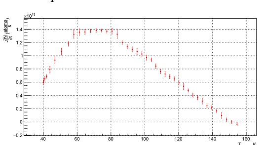
Dependence of the atomic beam intensity on the nozzle temperature, as measured at the outlet of the focusing system.
