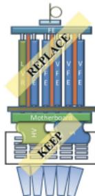
New VFE is designed with 30 ps precision for high energy signals
