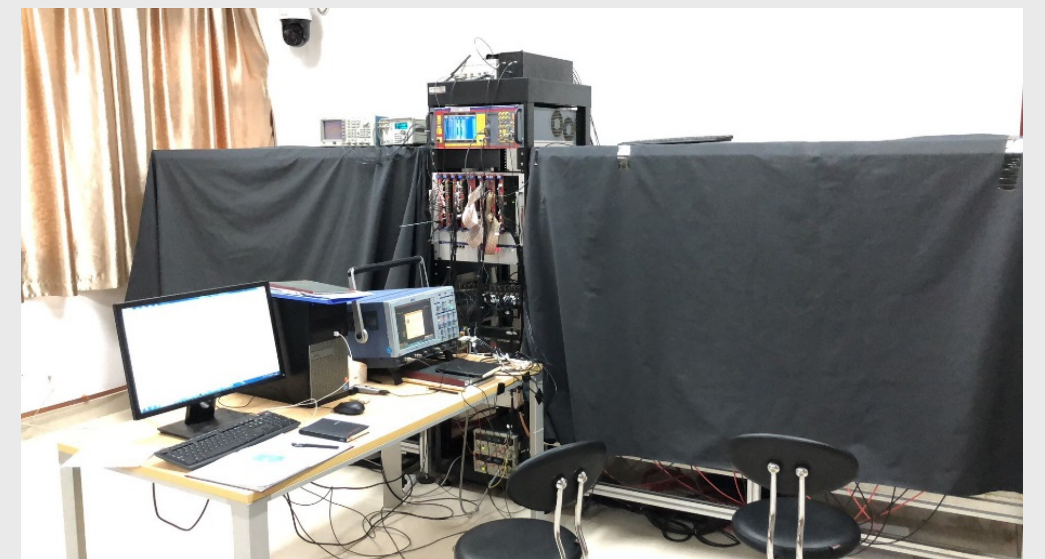
FIG. 5. PMT batch test system
