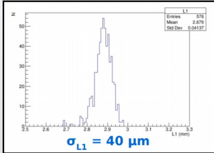
*Precision of the hole position vs corner of a cube*
