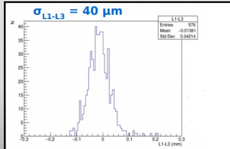
*Precision of hole position for two opposite sides of a cube. The main parameter that determines the angle of inclination of the hole*
