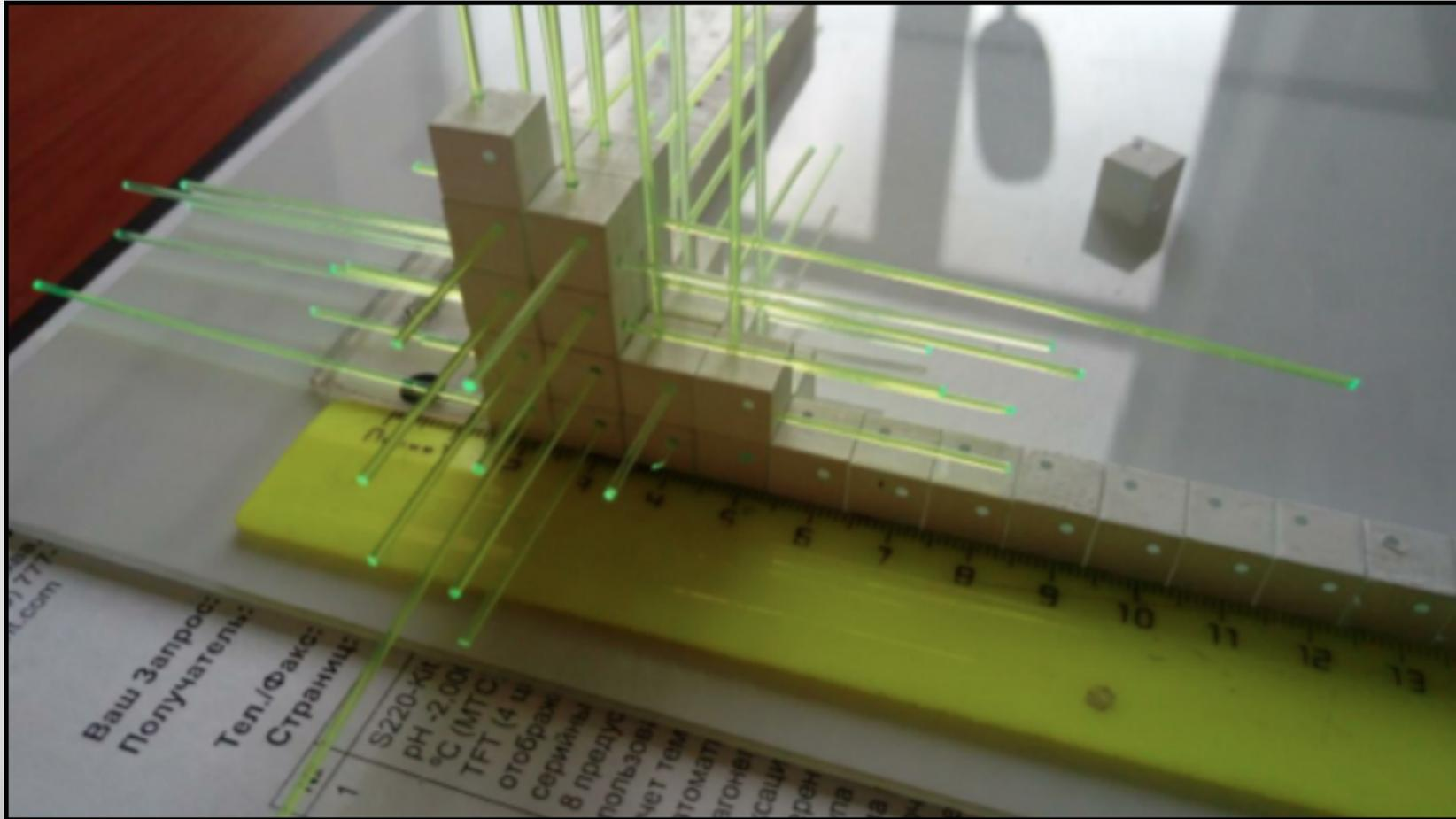
*The picture illustrates the readout method. A single WLS fiber is going through a row of cubes. One end of the fiber is viewed by a photosensor, another end is covered by a reflector. Each cube is viewed by 3 orthogonal fibers.*
