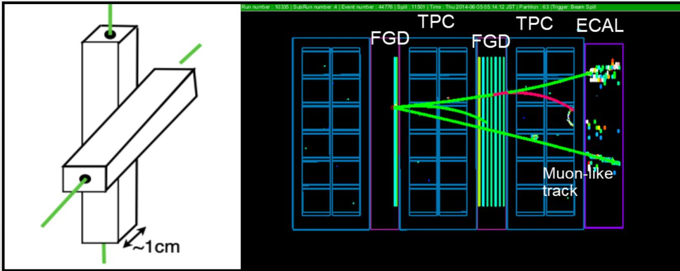
ND280 scintillator detectors (FGD) were designed as arrays of bars located perpendicular to the beam axis. Geometry is optimized to detect particles propagating in the forward direction that resulted in direction-dependence of acceptance and resolution for neutrino events.
