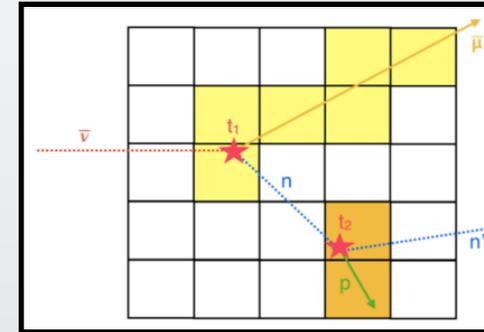
Example of the neutron detection through the observation of secondary protons
