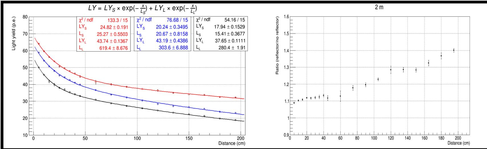
The single cube was flashed by LED. Fibers with/without reflector – red and blue line and with black paint on the end of fiber – black line.
