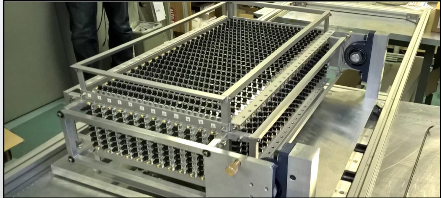
Two prototypes: **125** (5x5x5) cubes with **75** fibers and **9216** (48x24x8) cubes with **1728** was tested in the charge particles beam at CERN.
