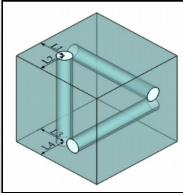
*For the full assembly of SuperFGD, the precision of a hole positions should be 40-50  $\mu\text{m}$*
