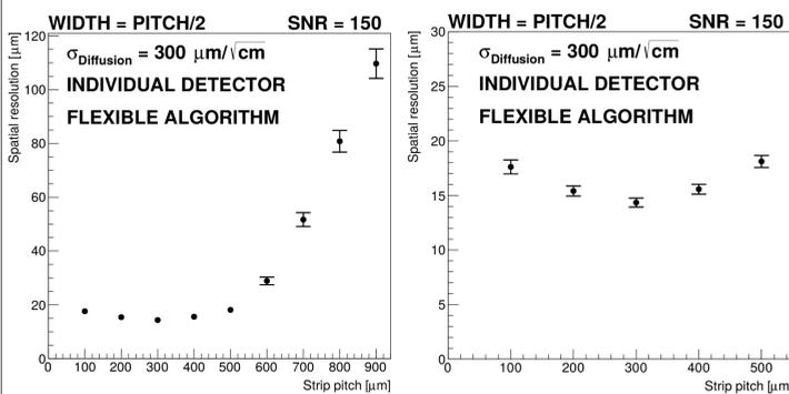
Fig. 2. Spatial resolution of individual triple-GEM detector in the simulation.
