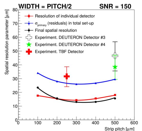
Fig. 4. Spatial resolution of triple-GEM detector within the complete set-up simulation in comparison with the experimental results.
