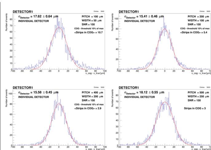
Fig. 1. Residuals distributions, obtained in the individual detector simulation.
