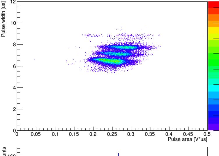
2D plot of pulse width versus pulse area and their axis projection spectra for alpha particles from <sup>233</sup>U (4.8 MeV), <sup>239</sup>Pu (5.2 MeV) and <sup>238</sup>Pu (5.5 MeV) source, measured in low-pressure TPC in isobutane at 120 torr and THGEM gain of 220
