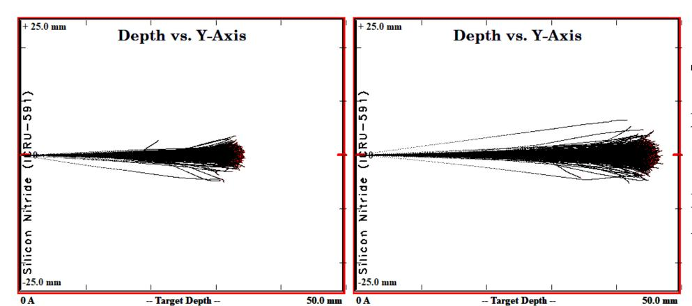
Tracks of <sup>10</sup>B and <sup>10</sup>Be respectively for 200 nm silicon nitride and 50 torr isobutane, obtained using the SRIM simulation
