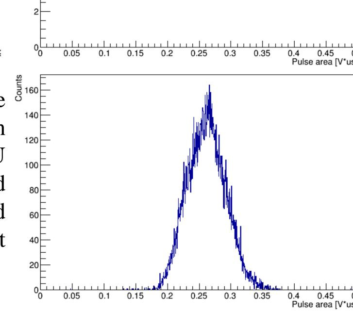
One can see that in low-pressure TPC the alpha particle lines can be effectively separated by pulse width (track ranges). On the other hand, these can hardly be separated by pulse area (energy).
