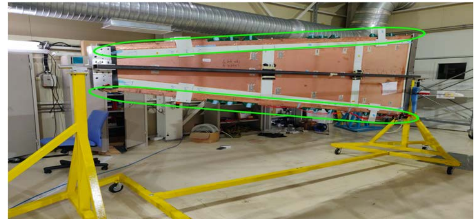
Completed Faraday cage
