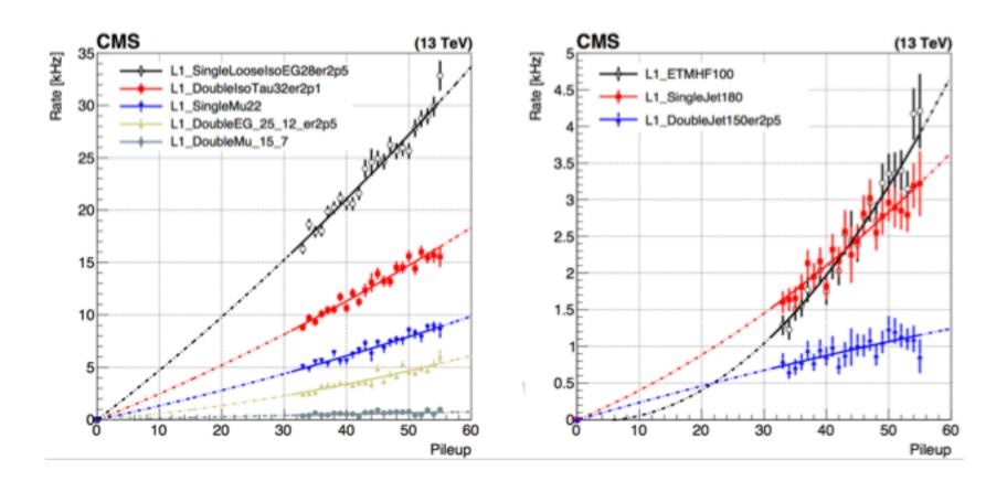
effect of higher pileup on trigger rates is in some cases much stronger than linear!
