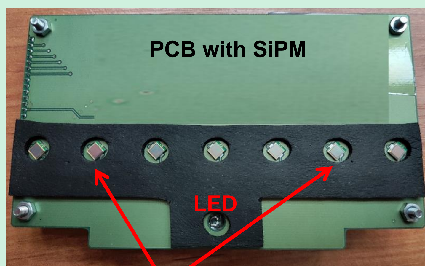
Hamamatsu MPPC S12572-010C/P with the pixel size 10x10 μm 2 .
