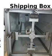
The detector is held from a central axis connected to its permaglass rings
