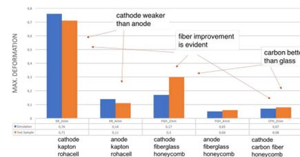
This choice, despite increasing the radiation length of the detector, was chosen because:
