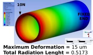
Maximum Deformation = 15  $\mu\text{m}$
