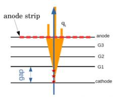
position reconstructed as average of the fired strips weighted by the charge on each strip
