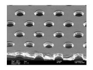
Polymeric kapton foil ( $T = 50 \mu m$ )
