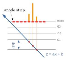
drift gap as a TPC gives the position of each ionization by the drift time and velocity → linear fit
