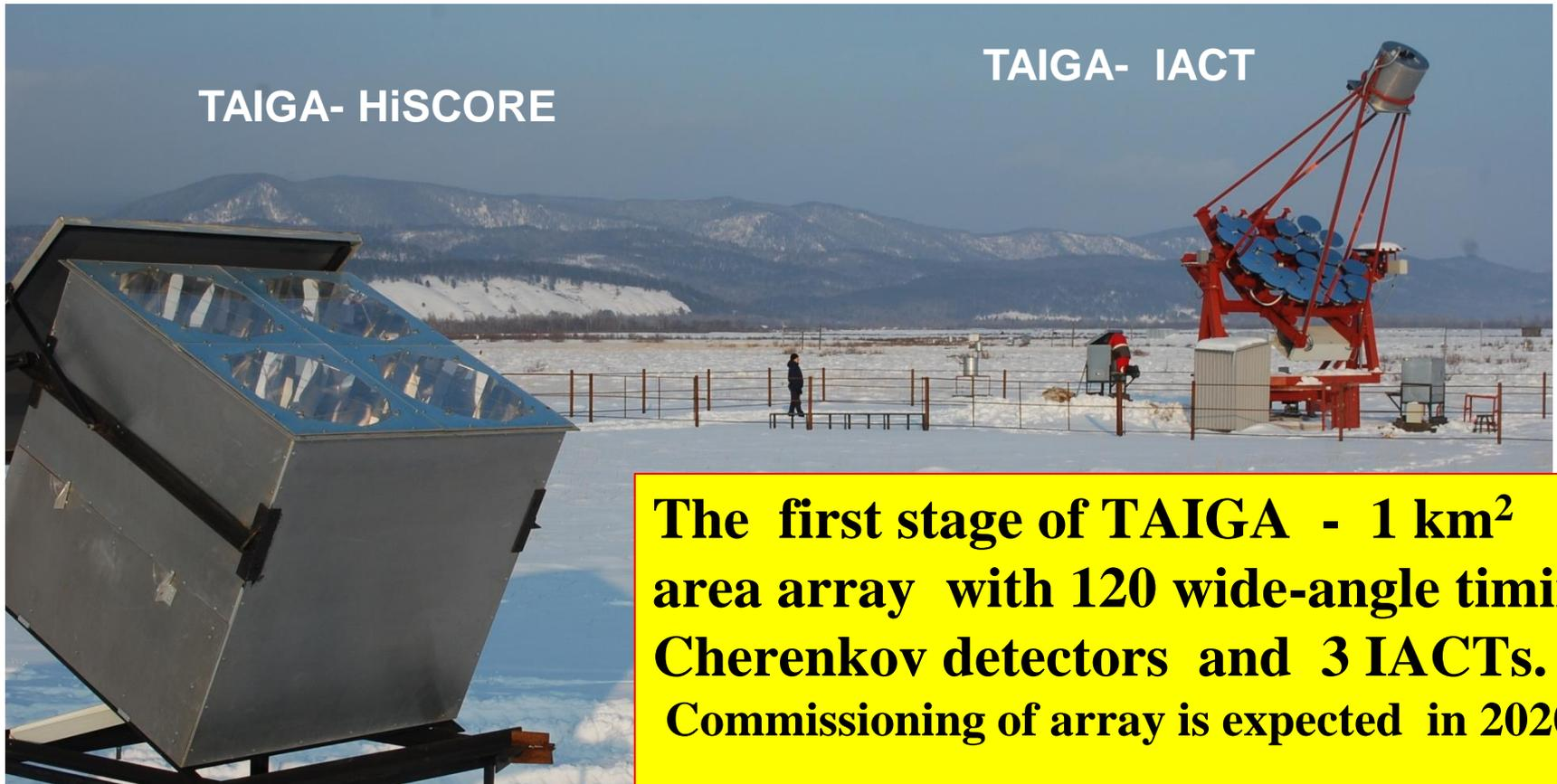
**The first stage of TAIGA - 1 km<sup>2</sup> area array with 120 wide-angle timing Cherenkov detectors and 3 IACTs. Commissioning of array is expected in 2020y.**
