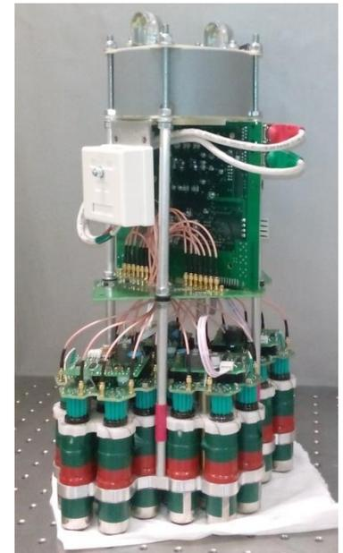
**Basic cluster: 28 PMT-pixels.** Signal processing:
