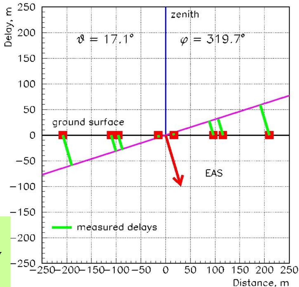
The **RMS=1.1 ns** for TAIGA-HiSCORE provides an accuracy of an  $\gamma$  and CR arrival direction about **0.1 degree**
