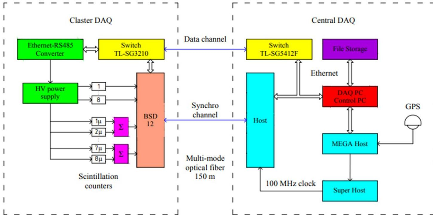
**Cluster DAQ** consists of a 12-channel data acquisition module (BSD-12), 2 ten-channel high-voltage power sources (HV power supply), a device for control of the high-voltage sources (Ethernet RS485 Converter), 4 two-channel analog signal summatoms ( $\Sigma$ ), and a Switch required for receiving and transmitting information.
