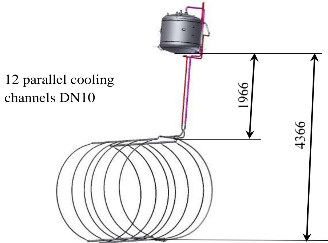
Liquid from the helium vessel of the Control Dewar will be fed through the forward pipeline and manifolds at the bottom of the support cylinder. From there, the liquid will be heated up in the tubes of the heat exchanger (a rib cage configuration) on the surface of the support cylinder.
