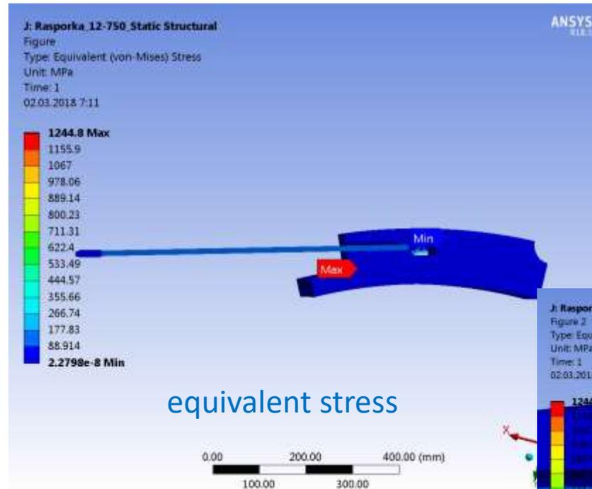
The equivalent stress of radial rods is ~120 MPa.
