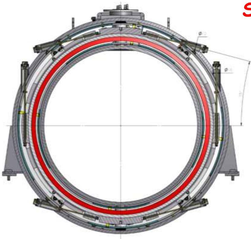
Cold mass is based into Cryostat with help suspensions and axis rods. Material of rods is Ti-5Al-2.5Sn
