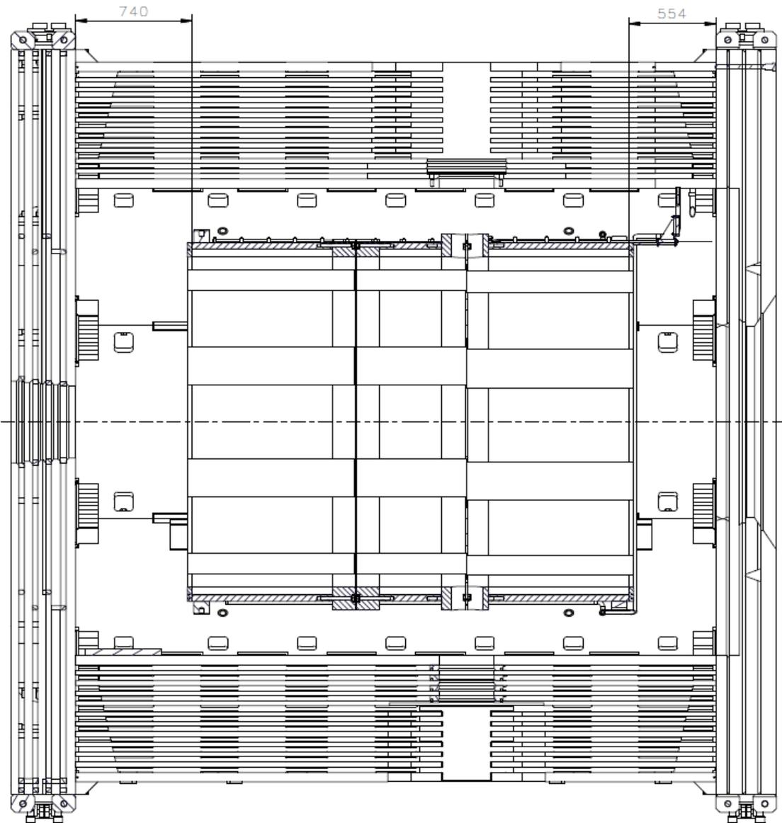
The maximal displacement of the Cold mass is 0,95 mm to upstream direction
