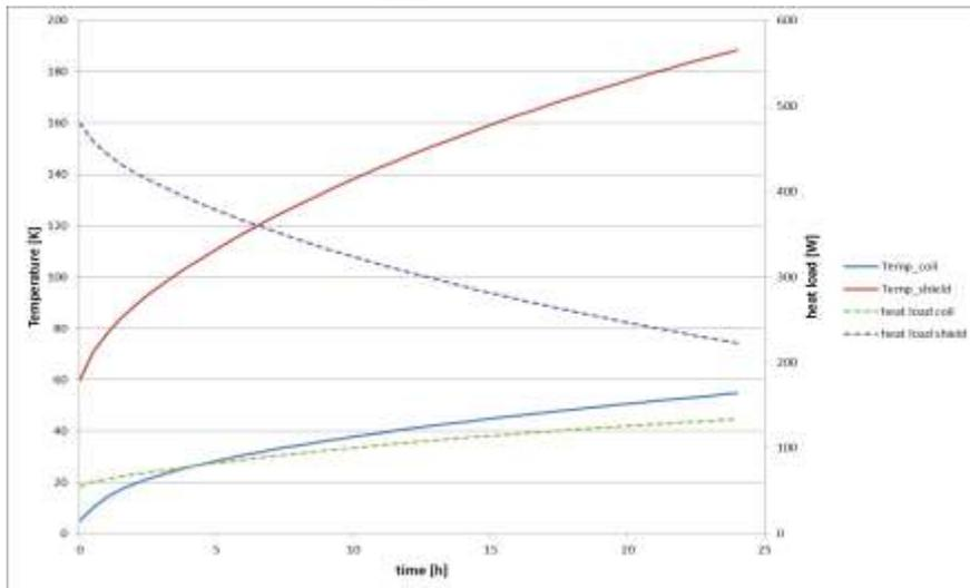
The maximal temperature of the thermal shield is estimated about 130K after 8 hours and the maximal temperature of the cold mass  $\approx 35$  K.
