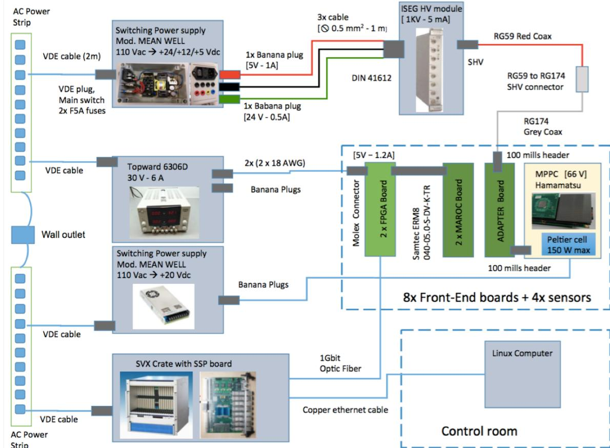
Each mRICH readout is completely independent of other modules in an mRICH array configuration.
