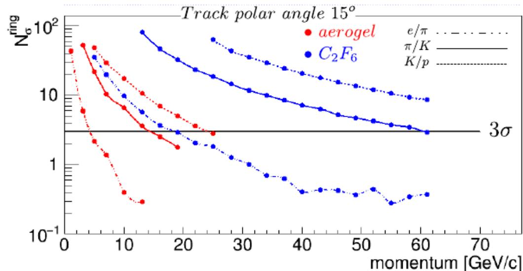
Hadron identification ( $\pi/K/p$ , better than 3 sigma from  $\sim 3$  up to  $\sim 50$  GeV/c for  $\pi/K$ )
