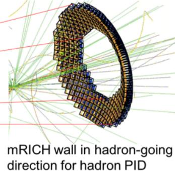
New features: a) separation of optical and electronic components; b) longer focal length (6"); c) 3mm x 3mm photosensors.
