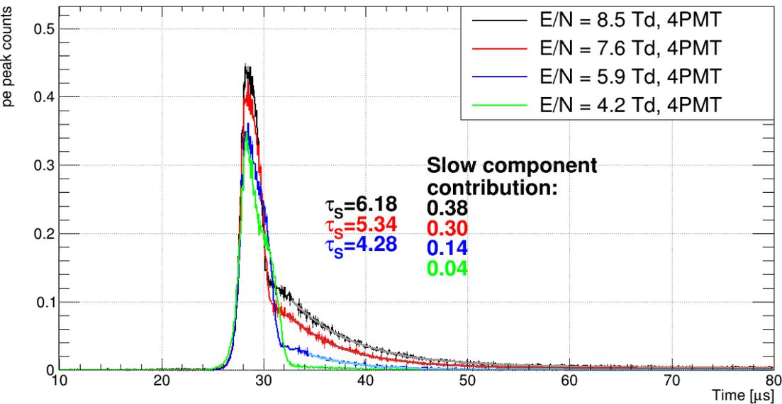
Results for SiPM-matrix (no WLS in setup), 88 keV  $\gamma$   $^{109}\text{Cd}$
