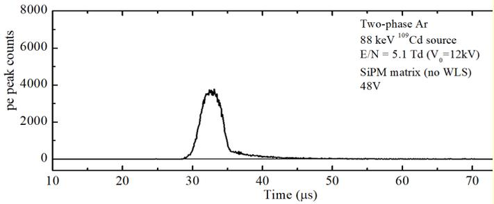
**Above the 4 Td EL threshold: SiPM-matrix data match the data without WLS**
