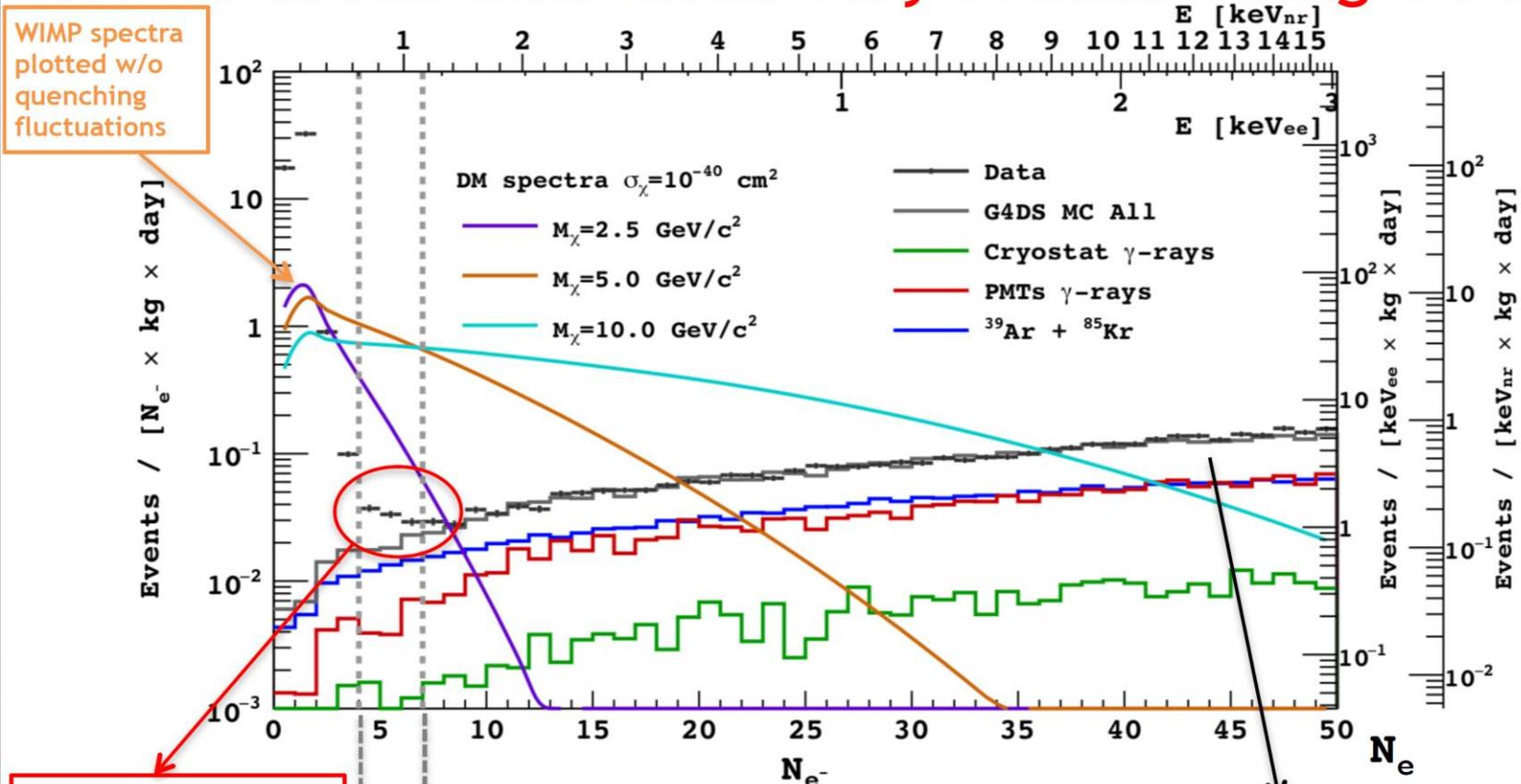
Excess of events wrt to background prediction due to trapped/delayed electrons peak.
