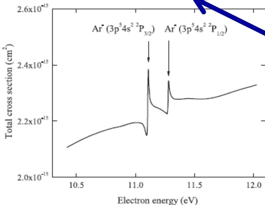
**Slow component in charge signal may appear if drifting electrons are delayed on metastable Ar<sup>-</sup> ions**
