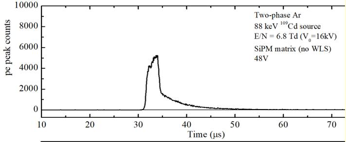
**PMT+WLS are different, have shape expected from excimer mechanism**
