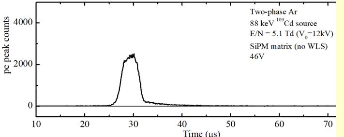
Just above the 4 Td EL threshold: slow component has emerged but fast component still dominates
