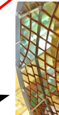
Mirror in the edge to increase photon detection efficiency.
