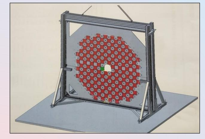
The detector is a cell structure hodoscope consisting of 280 scintillation counters. Each counter consist of scintillating tile with the size of 124x124x10 mm³ that is read by two groups of two SiPMs from the opposite sides. Two S14160-6050HS SiPMs from the same group are connected in series (for AC). The output signals from the groups are amplified (x30) and connected in analog "OR". Thus, each tile is read as a single electronic channel.
