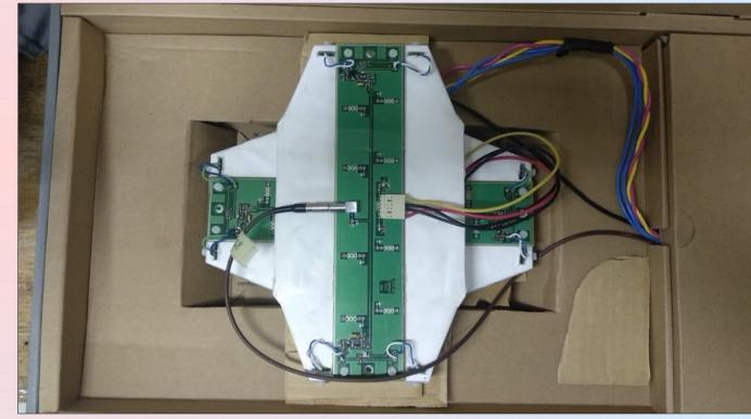
Since counters are identical, time resolution of individual counter could be estimated as  $\sigma = 310 / \sqrt{2} = 220$  ps.
