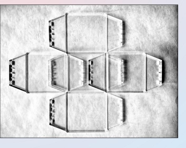
The tiles are fixed on both sides of aluminum frame in chessboard style with step of 120 mm, that makes 2 mm overlap of all neighboring counters.
