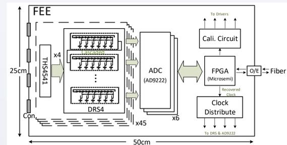
Fig. 3 The diagram of the FEE.
