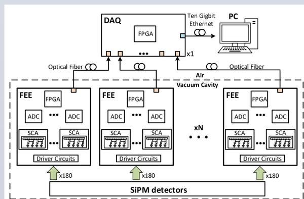
Fig. 2. Architecture of readout electronics system for the Gamma-Gamma collider.
