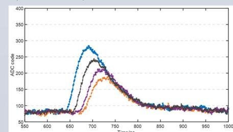
Fig. 8. Typical waveforms of the detector signal in one plastic scintillator strip.
