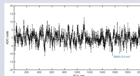
Fig. 5. Noise waveform of one channel on the FEE v1 after offset correction.
