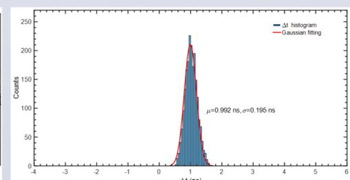
Fig. 6. Time interval histogram of the DRS4 SCA.
