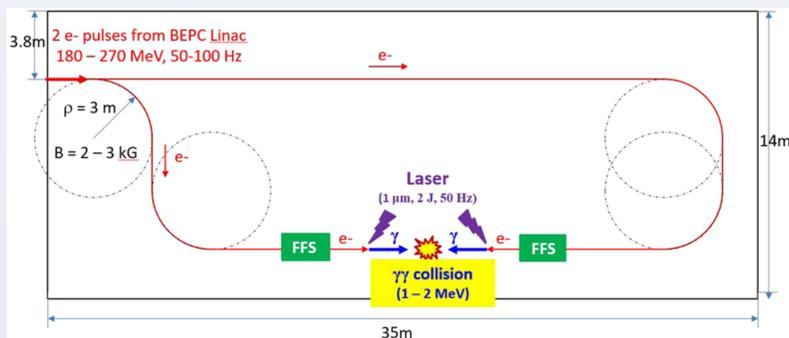
Fig. 1. A planned structure of the Gamma-Gamma collider facility.
