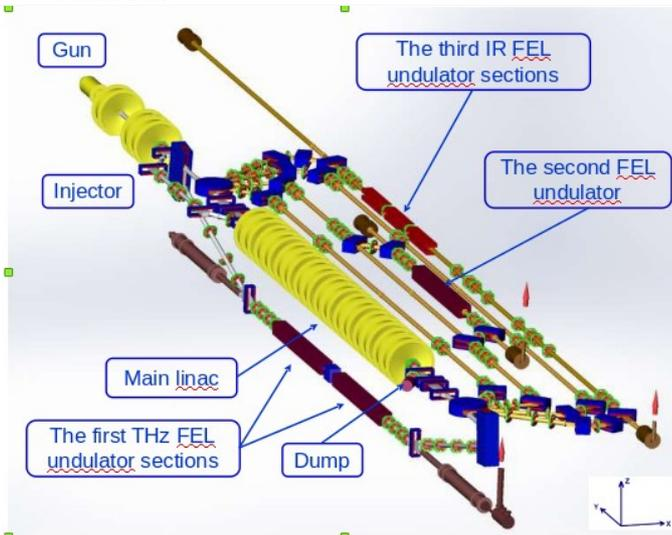
The Novosibirsk FEL of the terahertz and far-IR ranges is designed to generate narrow spectral lines with smooth continuous tuning of wavelengths from 5 to 240  $\mu\text{m}$  [1]. FEL is created based on the 40 MeV accelerator-recuperator.
