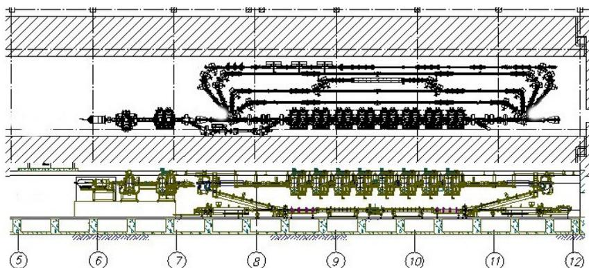
The distance between geodesic axes of 6 m, the height of the ground floor is 3.6 m.
