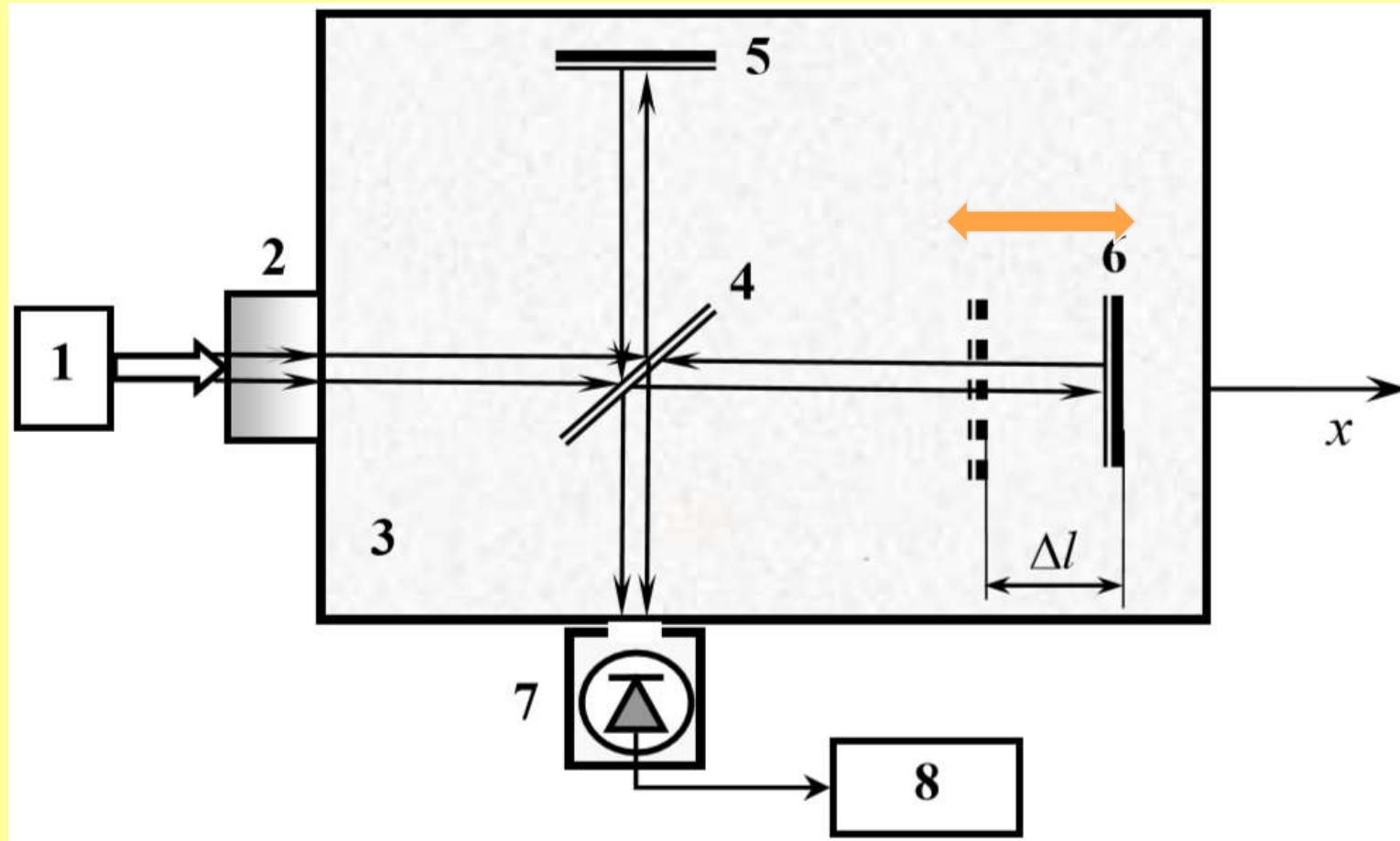
1 – broad-band THz radiation source; 2 – coupling element; 4 – flat plate beam splitter; 6 – discretely moving mirror; 7 - photo detector; 8 – computer.
