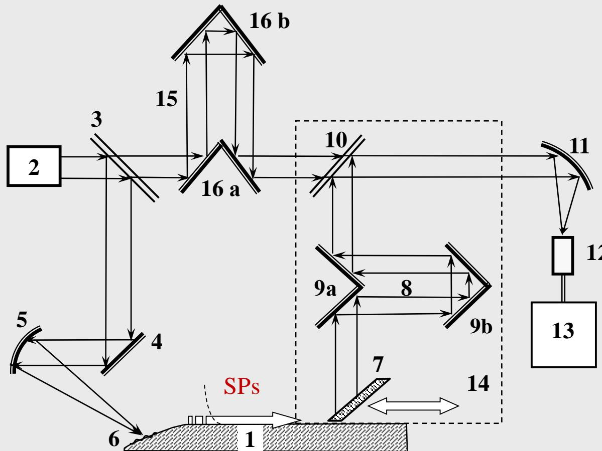
1 – sample; 2 – source of broad-band radiation; 3 - beam-splitter; 4, 5 – mirrors; 6 - coupling element; 7 – movable mirror, transforming SPs in bulk radiation; 8 – delay line; 9a – fixed corner mirror; 9 b – movable corner mirror; 10 - beam-splitter; 12 – photo detector, 13 – computer; 14 – movable platform; 15 – auxiliary delay line.
