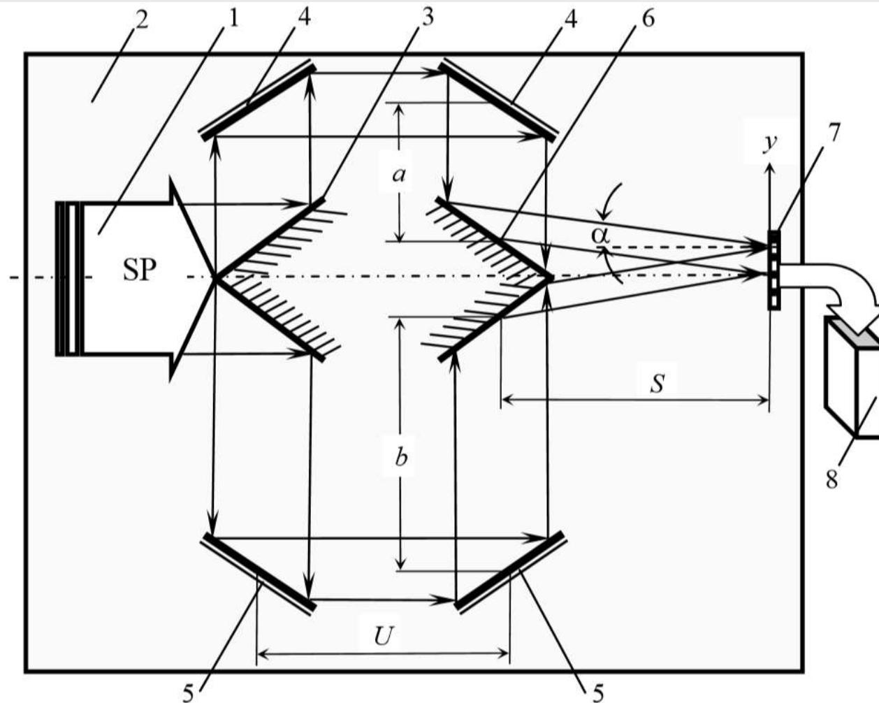
1 – initial SP beam; 3 and 6 – corner mirrors; 7 - array of photo detectors; 8 – computer.
