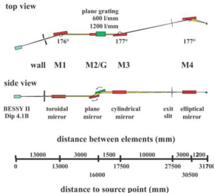
Usually, to implement methods where it is necessary to use the Soft X-ray range (15–2000 eV) the optical scheme is based on a monochromator with a plane grating and focusing mirrors.
