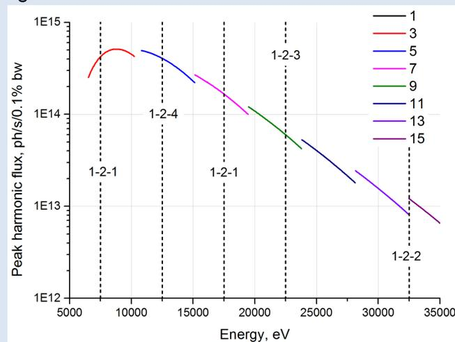
Undulator theoretical spectrum of SCU showing the first eight odd harmonics. The black dashed lines indicate the operation energy of all endstations in the primary mode (fixed energy). The solid lines show tunable energy for the 1-2-1 straight section in the alternative mode (all side branches are off).
