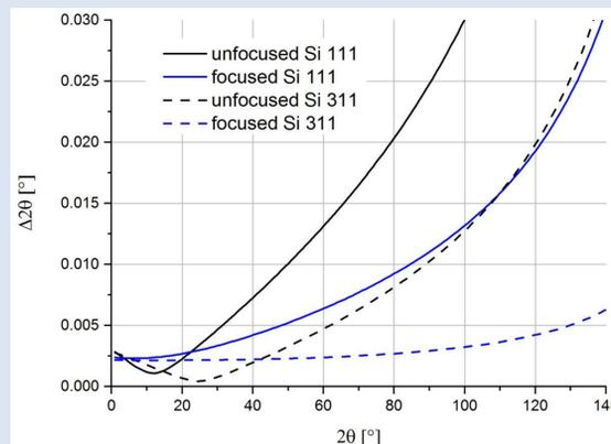
Theoretical curves of the instrumental resolution function for 1-2-1 working in the high-resolution mode at an energy of 17.5 keV when using Si (111) and Si (311) crystals (monochromator and analyser). Blue lines - with collimating (31 m) and focusing (41 m) CRL's, black - without focusing.
