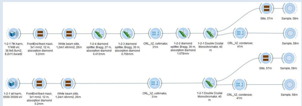
Optical scheme with the major optical elements of beamline 1-2-1 and the distances to the undulator source. Two branches shows two modes of operation (primary and with energy tuning).
