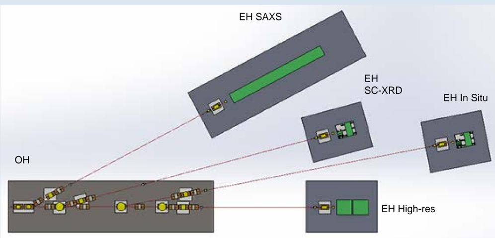
Beamline 1-2 setup, top view. Only optical (OH) and experimental (EH) hutches have shown. Optical elements (CRL's, monochromators, slits *etc.*) – yellow, endstations – green, granite bases – white.
