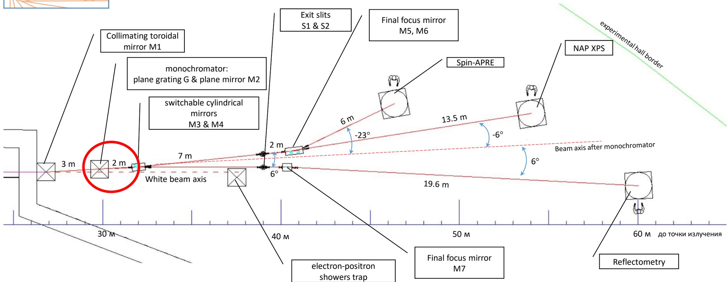
We use the so-called “collimated plane grating monochromator” optical scheme (cPGM). This scheme is based on the classic scheme of the SX-700 monochromator developed at the BESSY. The difference from the classical scheme is the presence of a collimating mirror M1 that turns a diverging beam to the parallel beam.
