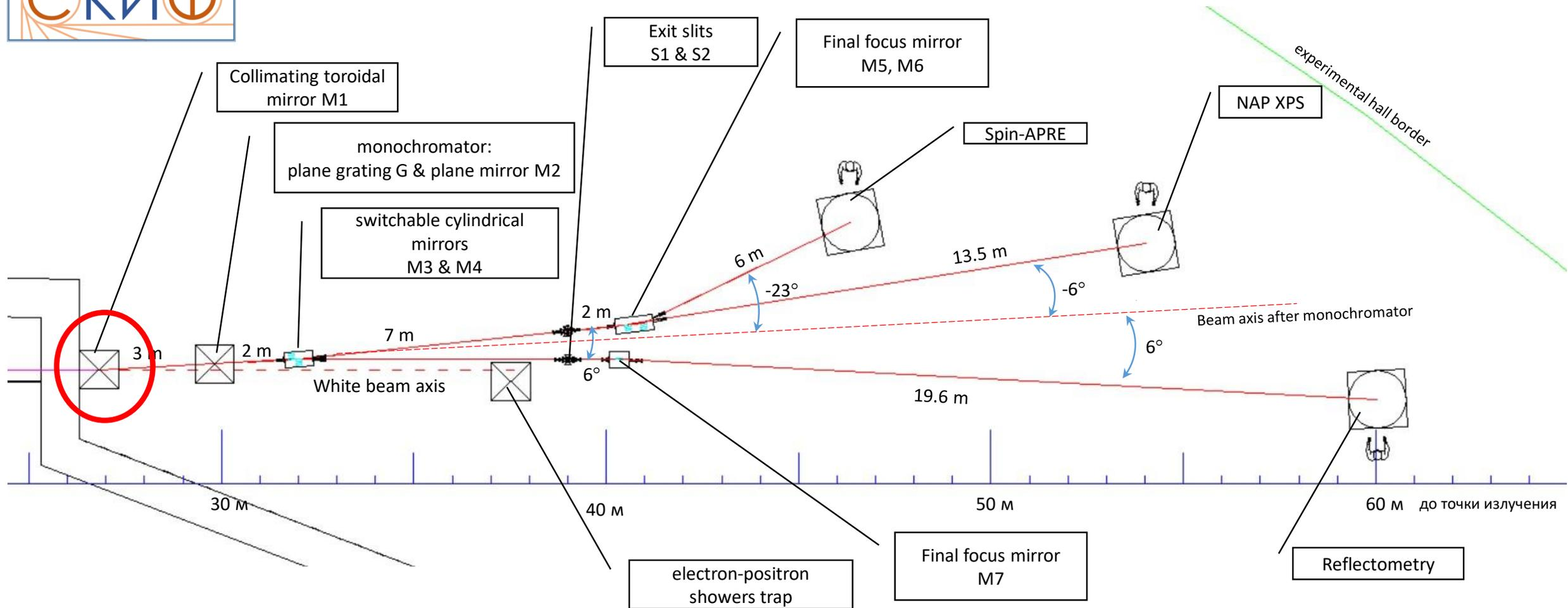
A collimating toroidal mirror. Installed immediately after the drive biosecurity wall (27 m from the radiation point). Focuses the beam horizontally on the slit (the distance from the mirror to the slit is 12 m). In the vertical direction it turns a diverging beam into a parallel beam for the collimated PG monochromator. The size of the working area of the mirror is 10 mm X 350 mm, therefore, the aperture of the captured beam is 6 X 10 mm<sup>2</sup> (width X height)
