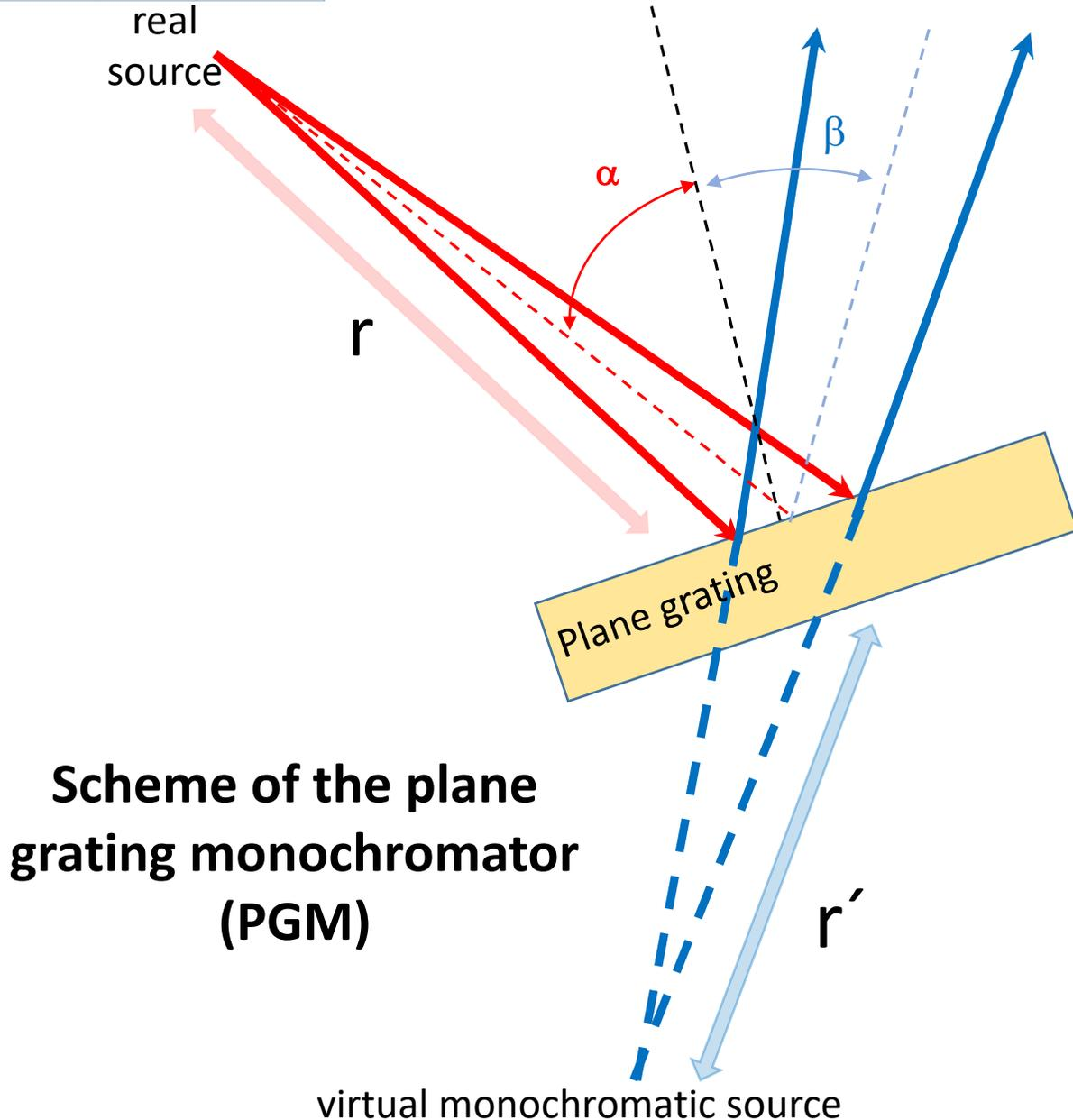
As is known, in the case of beam diffraction from a point source, a plane diffraction grating is a defocusing element, and the distance to the virtual monochromatic source  $r'$  obeys the rule
