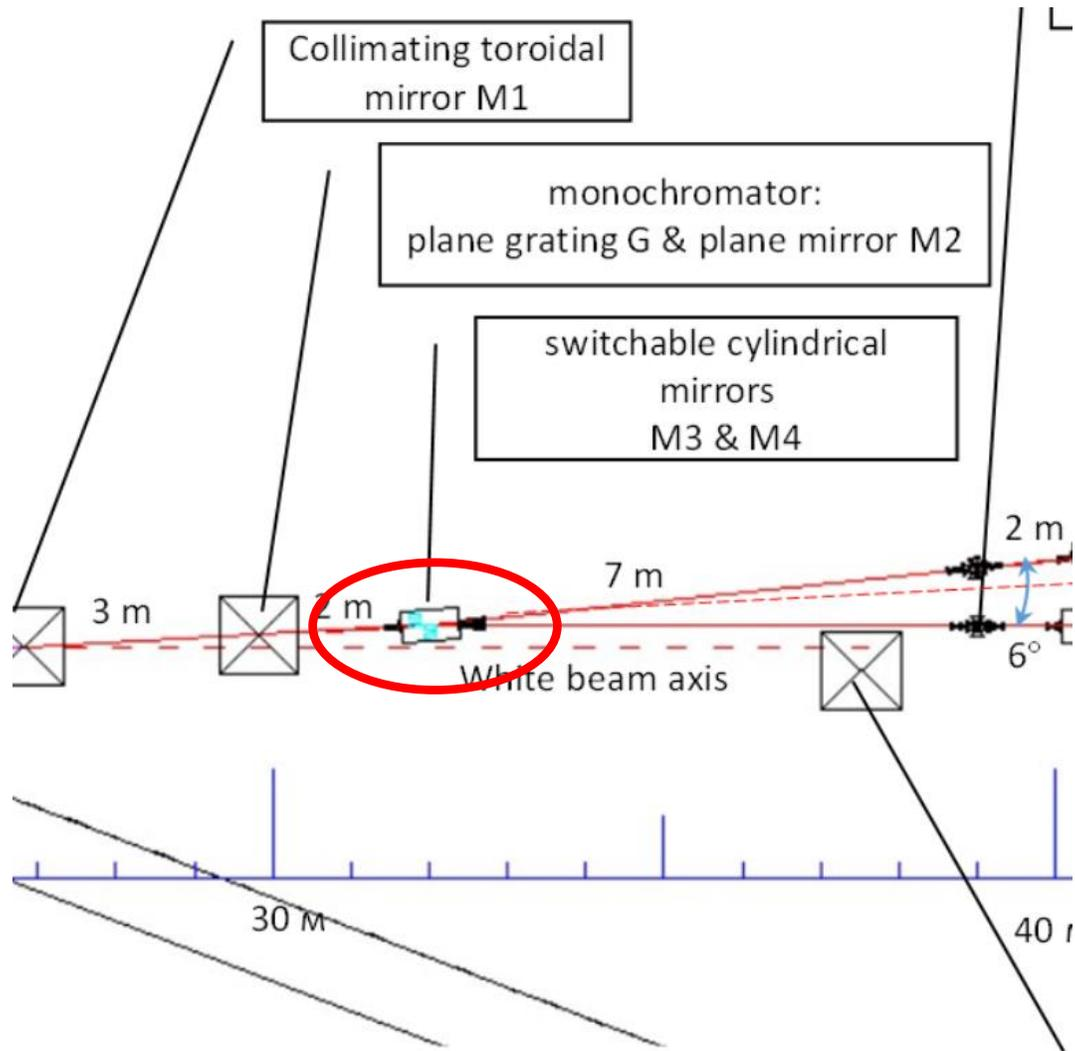
Two identical cylindrical mirrors focus the beam after the grating onto the exit slits of the monochromator S1 or S2 (distance 7 m). Mirrors are introduced into the beam alternately, installed at angles of  $+1.5^\circ$  and  $-1.5^\circ$ , deflect the beam by an angle of  $\pm 3^\circ$  in order to direct the beam to one of the three stations: "Metrology", Spin-ARPES or NAP XPS.
