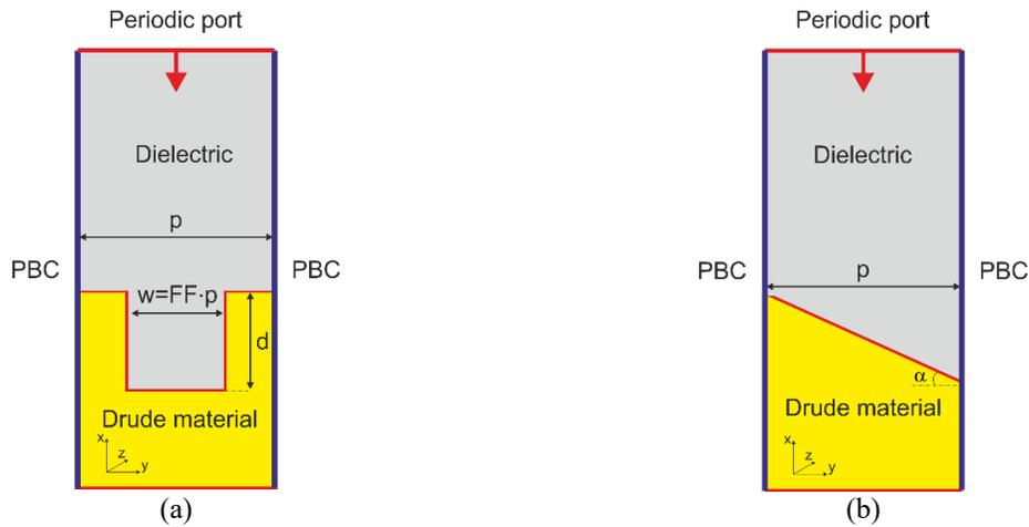
**FIGURE 2.** Floquet cell of (a) rectangular grating and (b) blazed grating.
