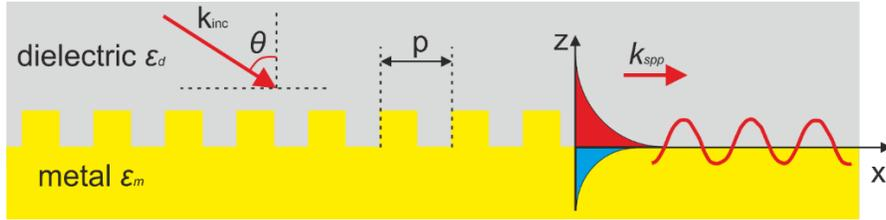
**FIGURE 1.** Schematic representation of the method of excitation of plasmon polaritons by grating coupling method.
