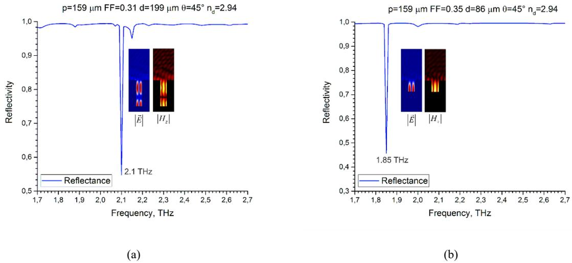
**FIGURE 6.** Optimal parameters of dielectric coated rectangular gratings.
