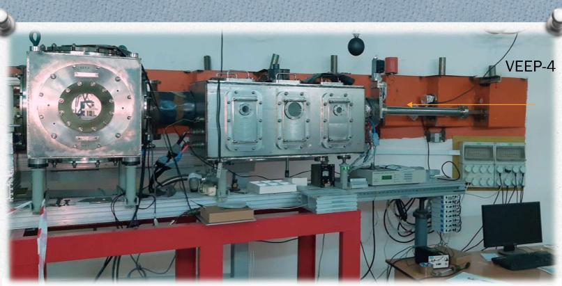
The *N10F* deflecting magnet at VEPP-4 storage ring is the source of radiation for the station. The electron energy in VEPP-4 was 4.5 GeV and magnetic field at point of radiation was 4.34 kG. The 4 beryllium foil of 200 microns each are installed in the beamline for vacuum protection of the storage ring.
