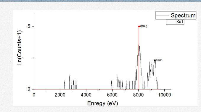
Spectrum calibration was performed in 2 iterations: First, the energy range of the fluorescent peak was determined based on the approximate position of the monochromator, then the center of the peak was taken as a point with the energy Ka of copper.
