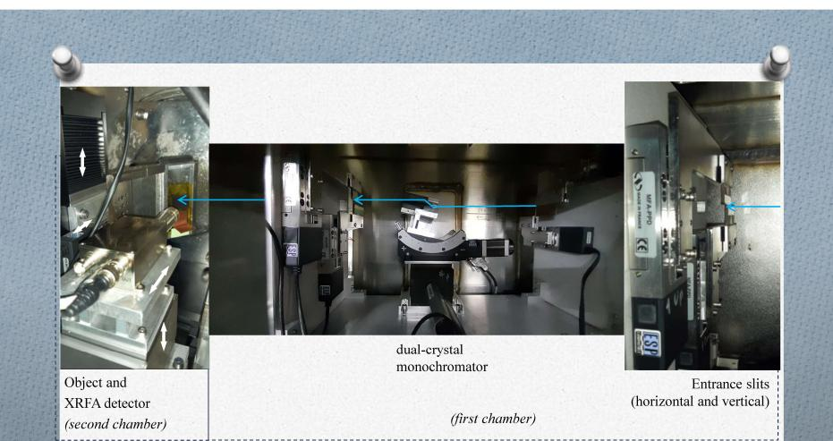
In the first test experiments, the method of x-ray fluorescence analysis using a silicon energy-dispersion detector was studied . The detector operated in 512 channel mode. The spectrum was shot for 180 seconds. In the chamber of the monochromator, the pressure was reduced to forevacuum. Copper foil was used as a test sample.
