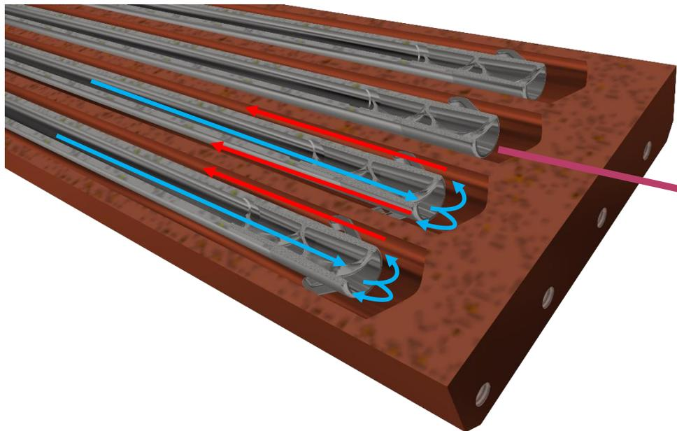
3x Anti-vibration springs on each Nozzle end
