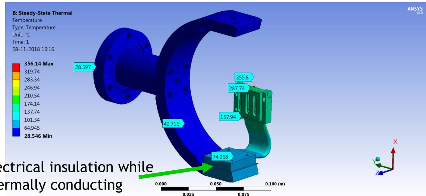
Electrical insulation while thermally conducting
