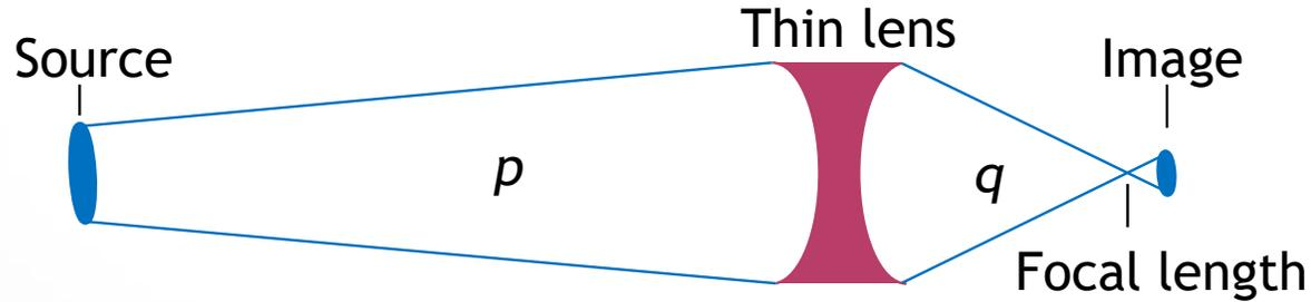
For a given beamline geometry the lens equation is fixed
