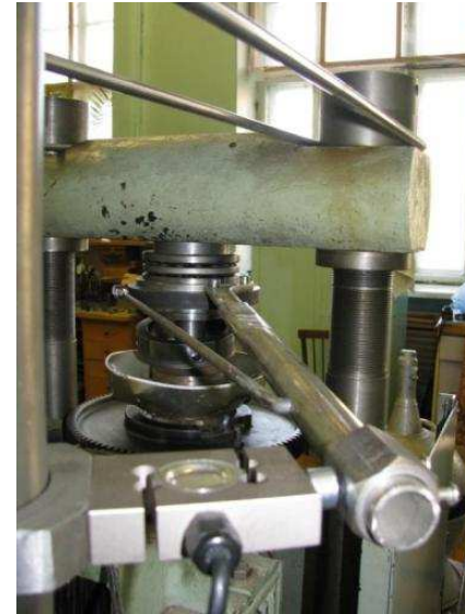
Fig. 1. The deformation scheme by the HPT method (a) and the image of the installation (b). F is the force produced by the hydraulic press; \omega - angular velocity of torsion of Bridgman anvil
