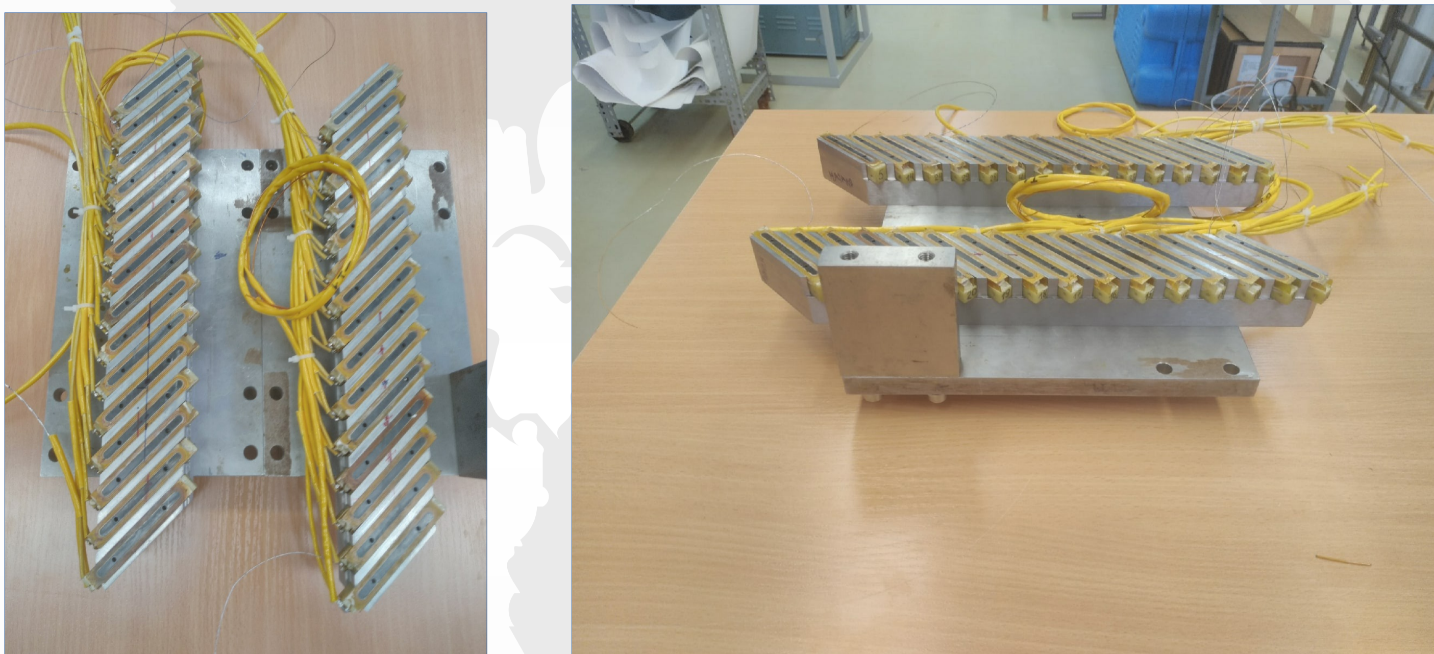
Figure 2: The prototype of a disassembled elliptical undulator. Upper and lower halves
