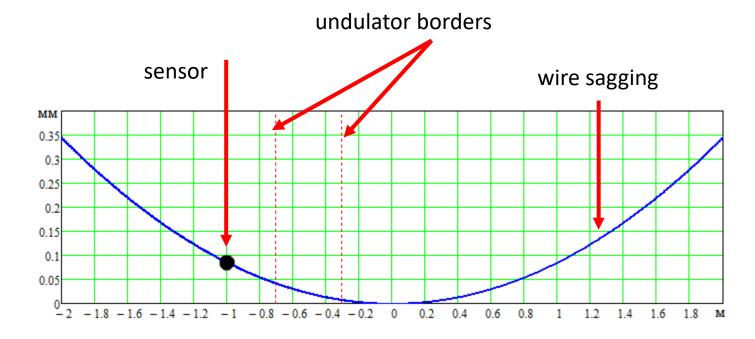
[Raw data from wire position sensor, brass wire  $Ø140 \mu m$ ]
