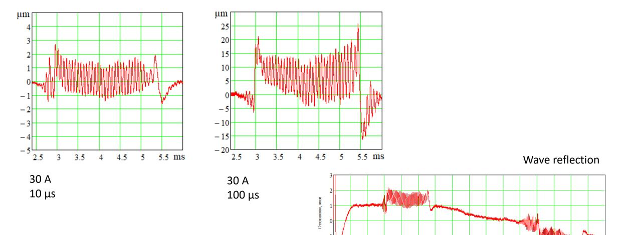
Время, мс [reconstructed, brass wire Ø140 μm, 30 A 10 μs pulse]
