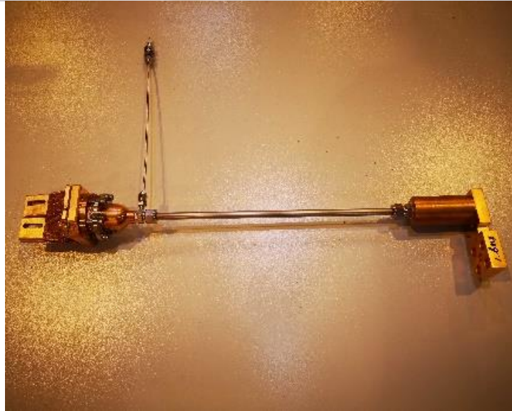
A recondenser (connected to 1 (60K) stage SRDK-415, an evaporator (mounted on a magnet) and a heat pipe assembly.
