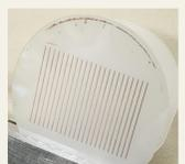
Fig. 6. Photo of an array for generation SPR fabricated in MEPhI Nanocenter
