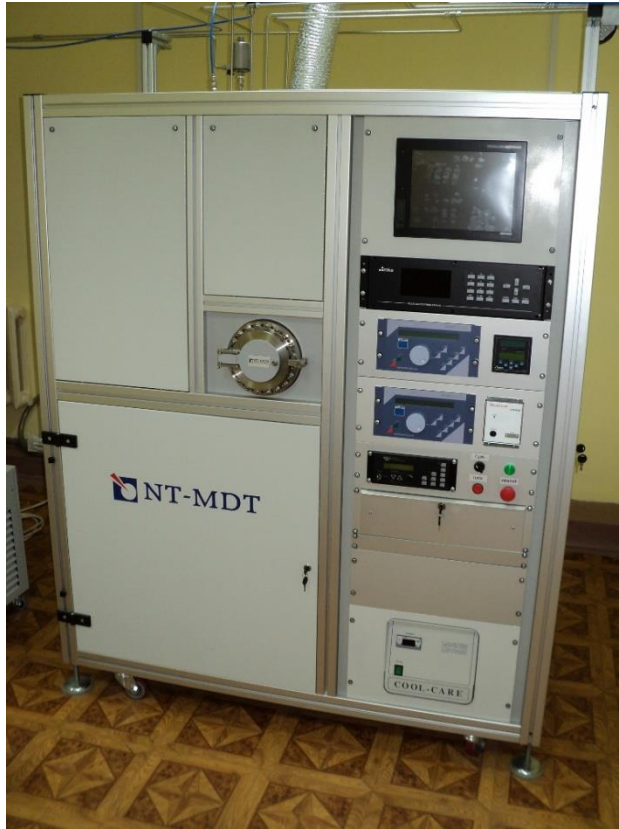
Plasma chemical etching system ETNA-100-PT produced by NT-MDT (Russia) in Samara University
