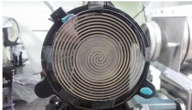
Realized diffractive optical element (Aperture diameter is 100 mm, wavelength is 129.5 \mu\text{m} )
