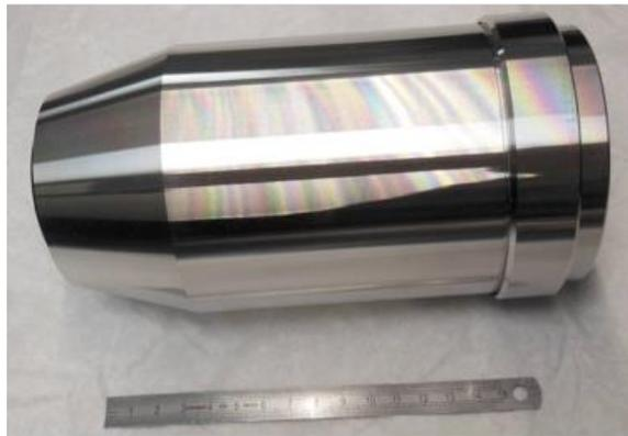
Front infinite correct objective (10 lenses)
