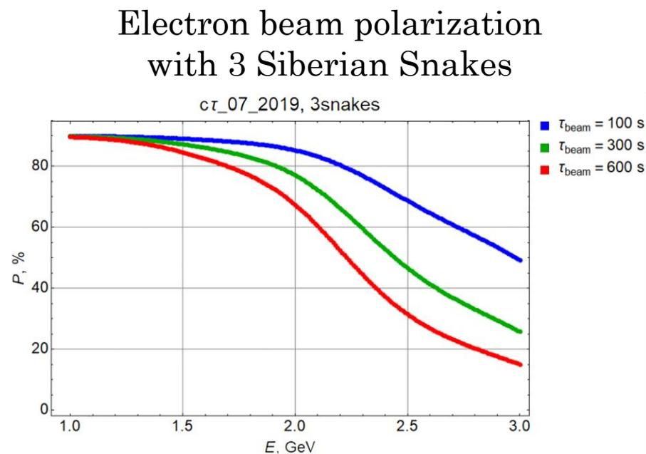
\* With two  $B_w = 3.5$  T wigglers that suppress intrabeam scattering
