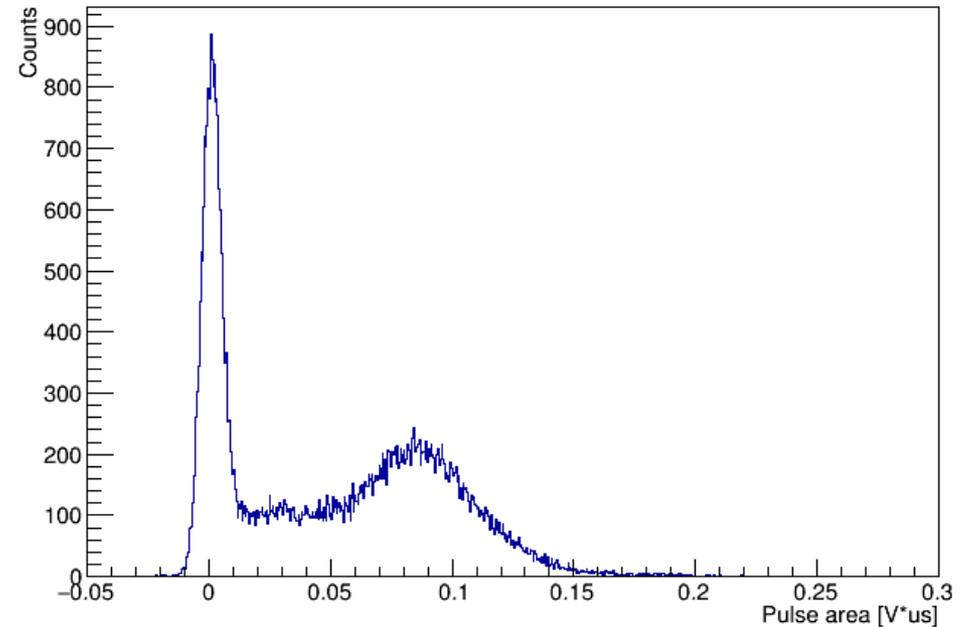
Pulse area spectrum of alpha particles from  $^{233}\text{U}$  (4.8 MeV),  $^{239}\text{Pu}$  (5.2 MeV) and  $^{238}\text{Pu}$  (5.5 MeV) sources from external part of the anode, measured in low-pressure TPC in Isobutane at 120 Torr
