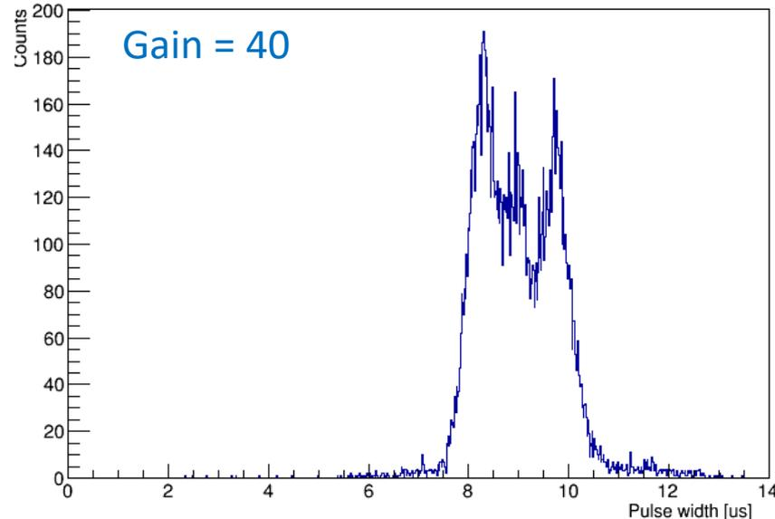
The lines of alpha particles are worse separated with less effective gain of THGEM and longer shaping time of amplifier
