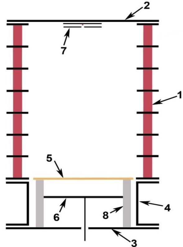
TPC construction: 1 – field shaping rings, 2 – removable top flange, 3 – removable bottom flange, 4 – transitional gap, 5 – THGEM, 6 – sectioned anode, 7 – alpha particle source, 8 – caprolon rods
