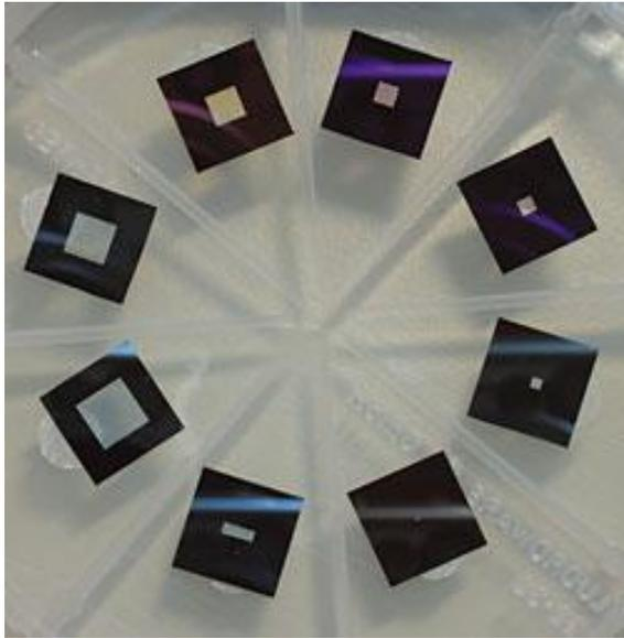
Figure of silicon nitride membrane windows
