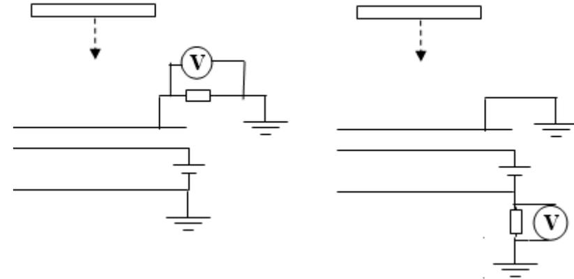
The scheme of effective gas gain measurement
