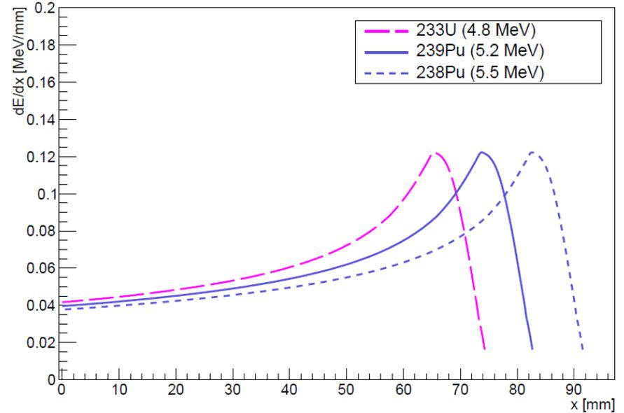
Energy loss as a function of distance in Isobutane for alpha particles with different energy at 120 Torr
