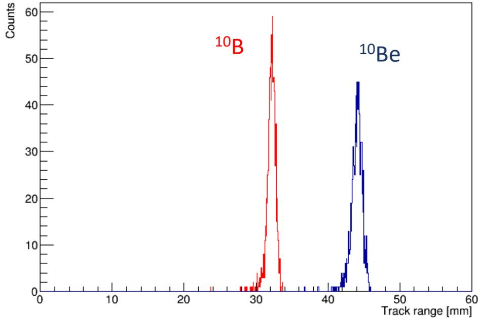
Spectra of track ranges for  $^{10}\text{B}$  and  $^{10}\text{Be}$  with energy 4.025 MeV in 200 nm silicon nitride and Isobutane at 50 Torr
