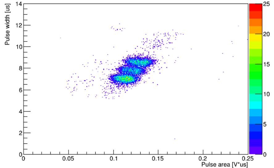
2D plot of pulse width versus pulse area and their axis projection spectra for alpha particles from  $^{233}\text{U}$  (4.8 MeV),  $^{239}\text{Pu}$  (5.2 MeV) and  $^{238}\text{Pu}$  (5.5 MeV) source, measured in low-pressure TPC in Isobutane at 120 Torr and THGEM gain of 40. The pulse width and pulse area spectra reflect those of the track range and energy.
