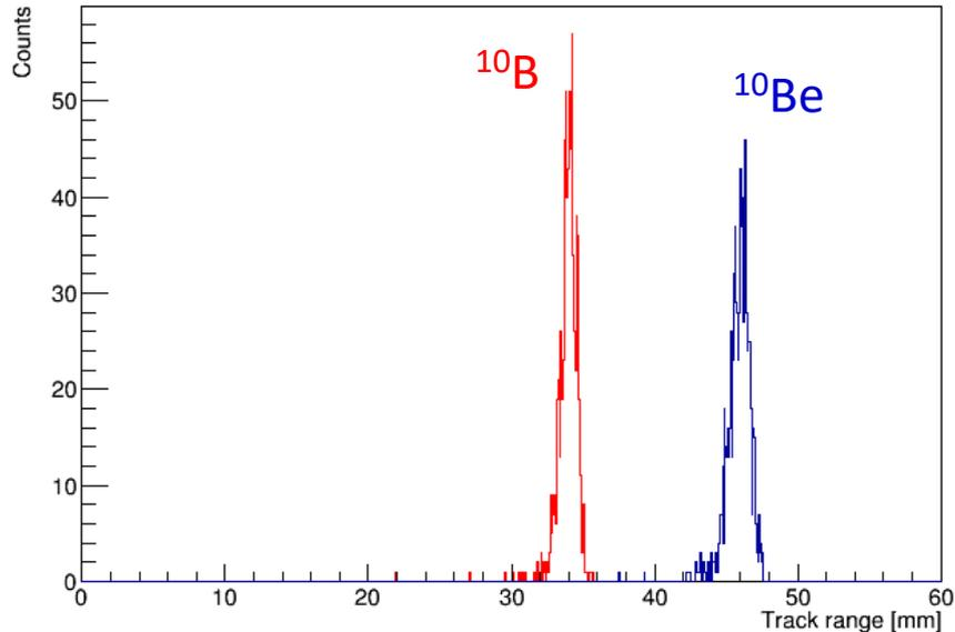
Using these results and SRIM code simulation, we see that the isobaric boron and beryllium ions (having range difference of 32%) can be effectively separated at the level exceeding 10 sigma
