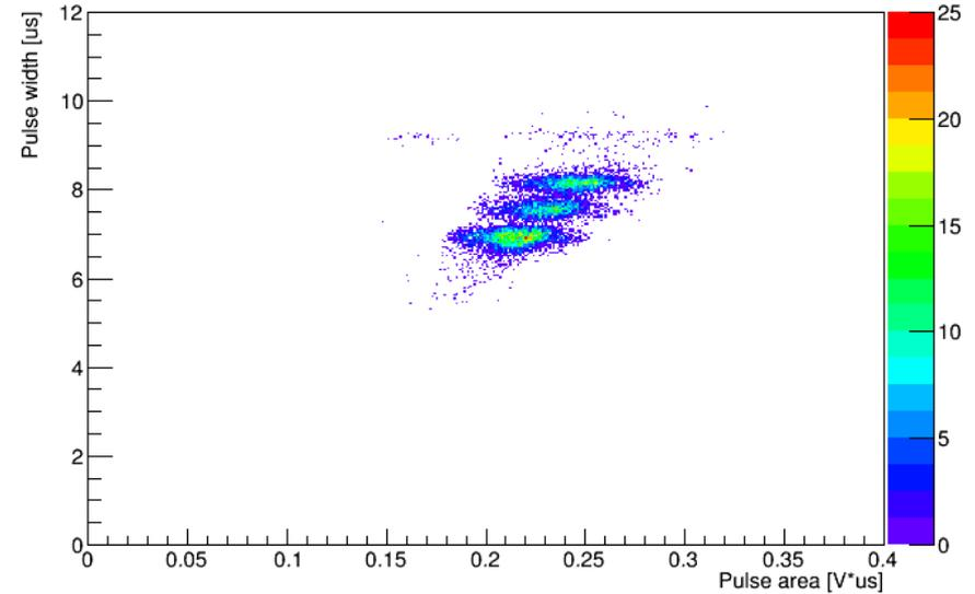
2D plot of pulse width versus pulse area and their axis projection spectra for alpha particles from  $^{233}\text{U}$  (4.8 MeV),  $^{239}\text{Pu}$  (5.2 MeV) and  $^{238}\text{Pu}$  (5.5 MeV) source, measured in low-pressure TPC in Isobutane at 120 Torr and THGEM gain of 60. The pulse width and pulse area spectra reflect those of the track range and energy.
