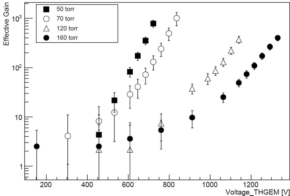
THGEM effective gain as a function of the voltage in Isobutane at pressures varying from 50 to 160 Torr in the low-pressure TPC
