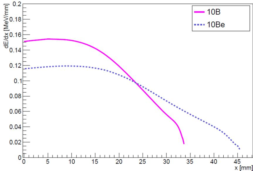
Energy loss as a function of distance in Isobutane for  $^{10}\text{B}$  and  $^{10}\text{Be}$  with an energy of 4.025 MeV at 50 Torr
