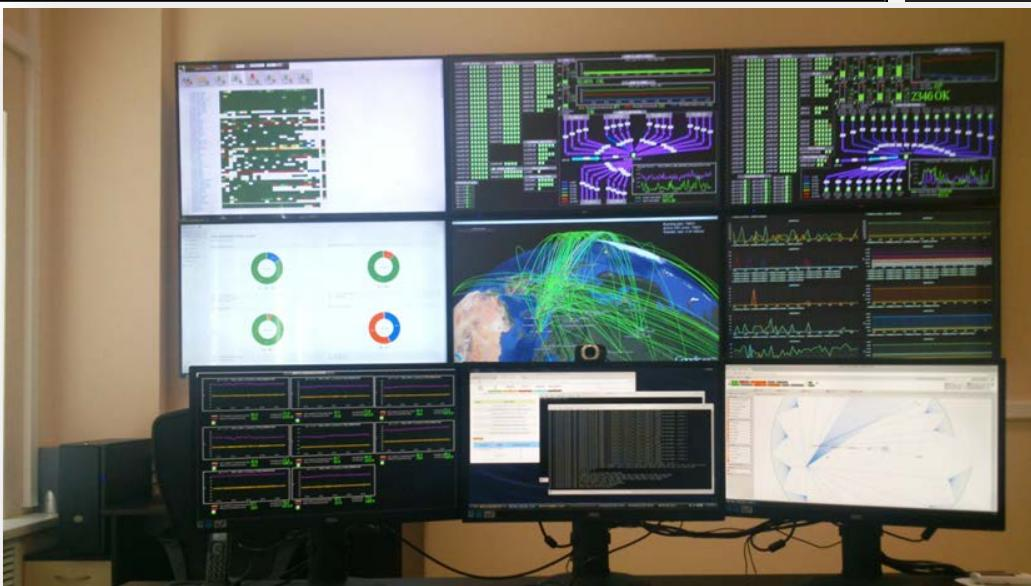
The system allows one, in a real time mode, to observe the whole computing complex state and send the system alerts to users via e-mail, sms, etc. ~ 850 elements are under observation
