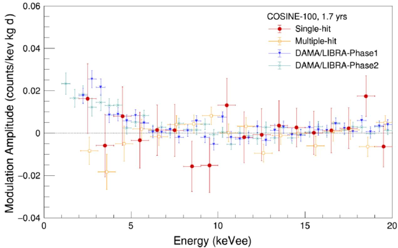
FIG. 5. Modulation amplitude as a function of energy in 1 keV bins for the 1.7 year COSINE-100 single-hit (red closed circle) and multiple-hit (orange open circle) events. DAMA/LIBRA phase 1 (blue) and phase 2 (green) from Ref. [12] are also shown
