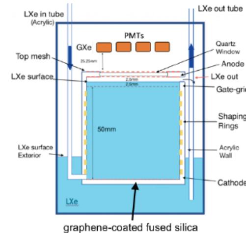
LBECA prototype - sealed chamber with high chemical purity
