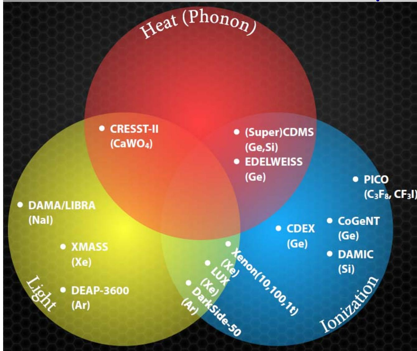
To discriminate the dark-matter signal from background processes, one exploits one or two out of three possible signals: heat (phonons), scintillation light (photons) and ionization (electrons).
