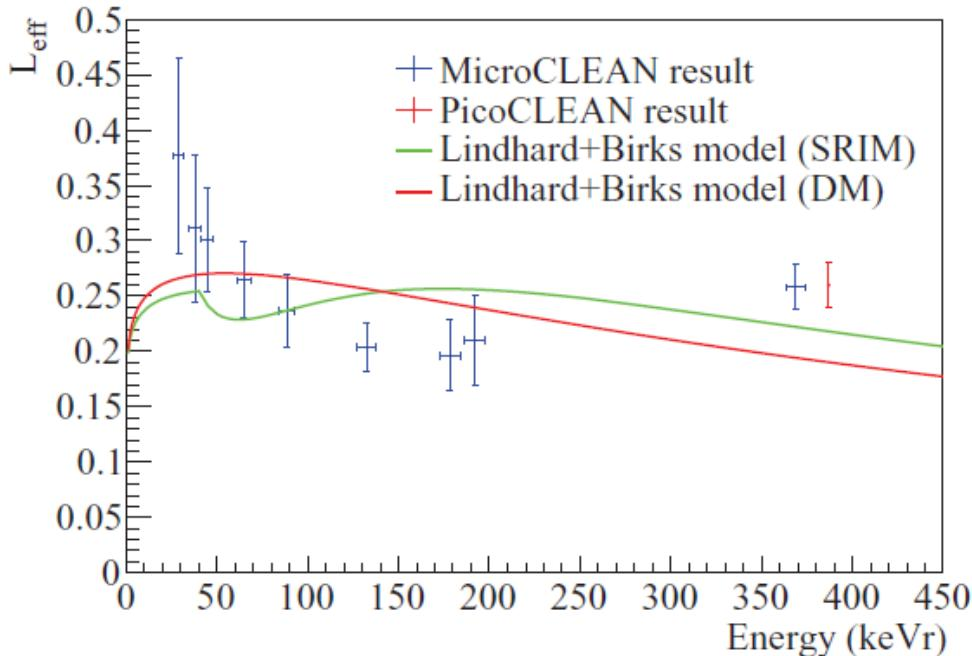
**FIG. 13.** (Color online) The observed nuclear recoil scintillation efficiency vs nuclear recoil energy in neon, along with the Lindhard + Burks model described in the text.
