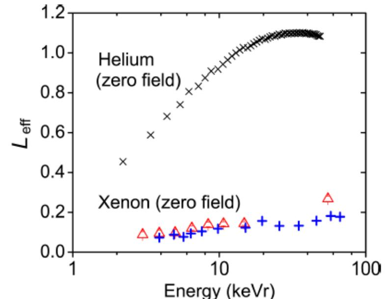
**FIG. 11:** (color online) The effective quenching factor  $L_{eff}$  as a function of the recoil event energy. The  $\times$  represents the calculated  $L_{eff}$  for helium under zero applied electric field. The measured data for liquid Xenon by G. Plante *et al.* [88] ( $\Delta$ ) and by A. Manzur *et al.* [89] ( $+$ ) are also shown.
