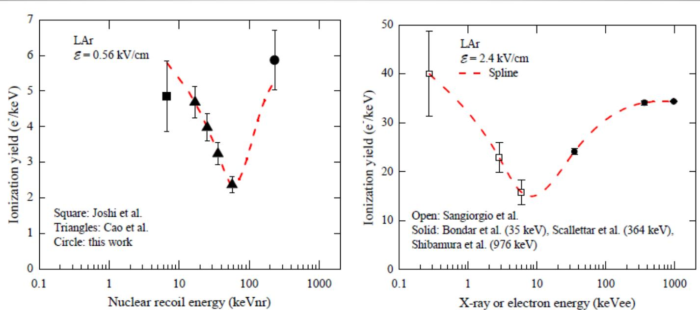
**Figure 6.** Ionization yield of nuclear recoils in liquid Ar at 0.56 kV/cm as a function of the energy, measured in Joshi et al. [5], Cao et al. [6] and this work. The curve is drawn by eye.
