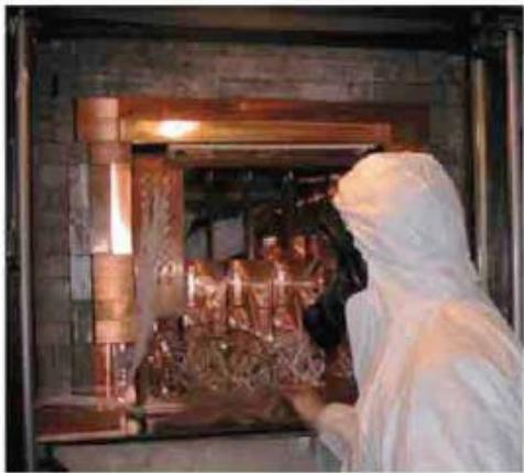
As a result of a 2nd generation R&D for more radiopure NaI(Tl) by exploiting new chemical/physical radiopurification techniques (all operations involving - including photos - in HP Nitrogen atmosphere)
