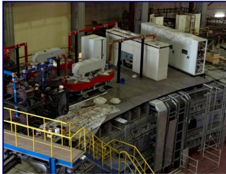
**Booster PSs placed on the top of the Synchrotron yoke**
