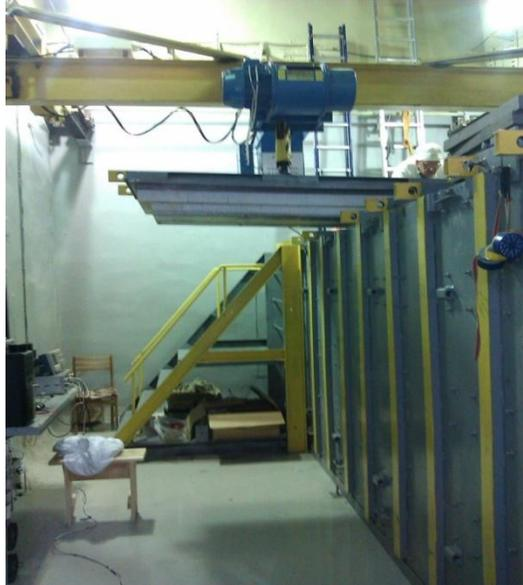
Passive shielding - 60 tons
