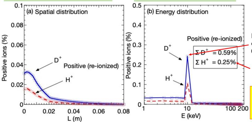
Particles in peak energy in 0.25% for D, 0.1% for H.
