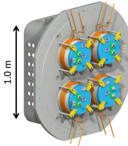
**Size scaling: half ITER source size experiment (100×90 cm<sup>2</sup>)**
