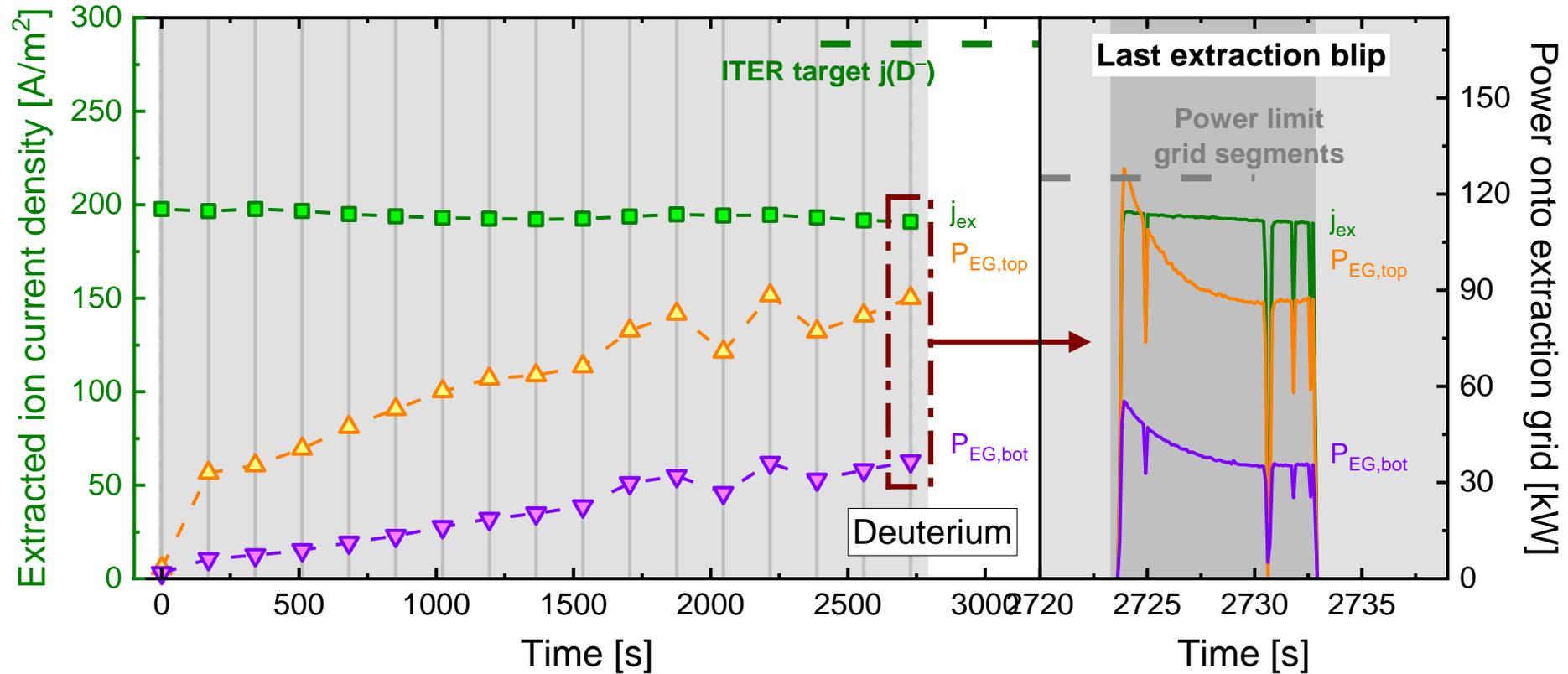
**Co-extracted  $e^-$  during best long pulses in  $D_2$  at  $p_{fill}=0.3$  Pa up to now ( $\approx 67\%$  of current density target):**
